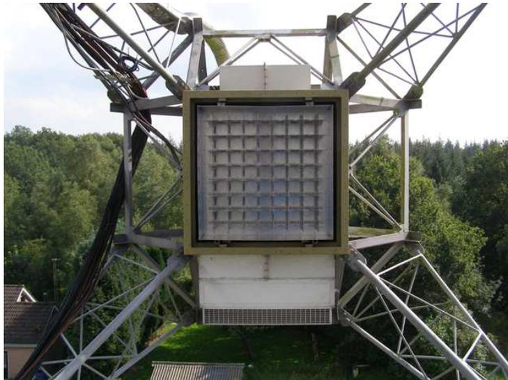
Figure 1.4: One of the FPA prototypes positioned in the Westerbork Synthesis Radio Telescope.
