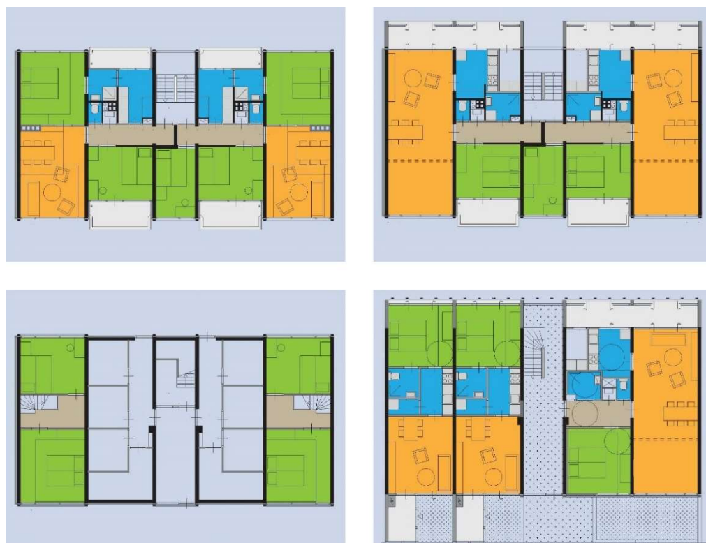
Figure 6. VAM walk-up apartment building (1960) with type E3 floorplan. Top left: original plan 2e, 3e, and 4e floors. Bottom left: original ground floor. Top right: new plan 2e, 3e, and 4e floors. Bottom right: new plan ground floor. Drawing Leo Oorschot.
