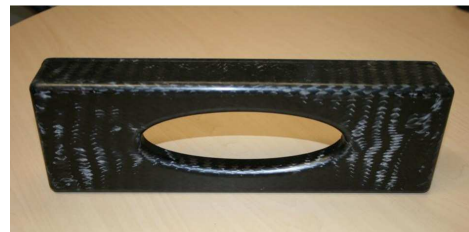
Figure 6: Manufacturing of one of the longitudinal beam by vacuum and one part of the transversal beams by hand lay up.
