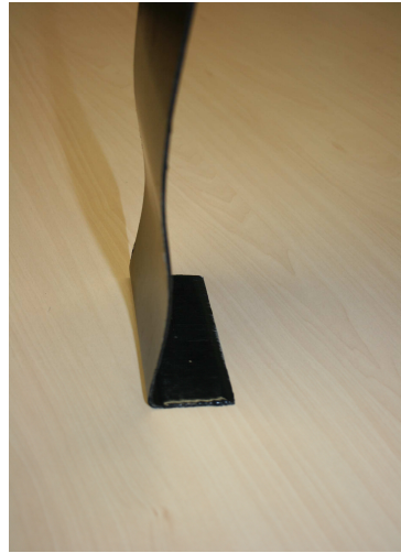
Fig 11: Positive mould of the exterior side body panels and a sample of IXIS strip shaped to the contour of 5th door of Superbus
