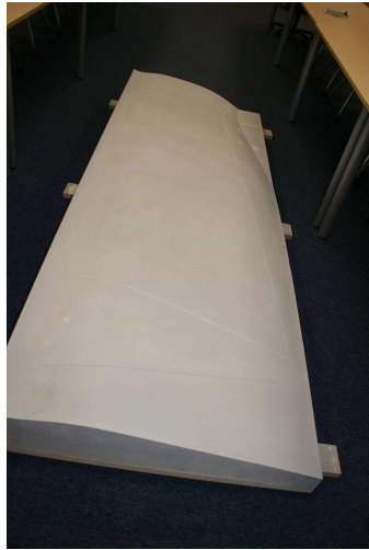
Fig 11: Positive mould of the exterior side body panels and a sample of IXIS strip shaped to the contour of 5th door of Superbus
