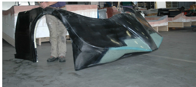
Figure 10: Nose of the vehicle. All carbon fiber apart from some areas in glass fiber (light blue) required for radars functioning.
