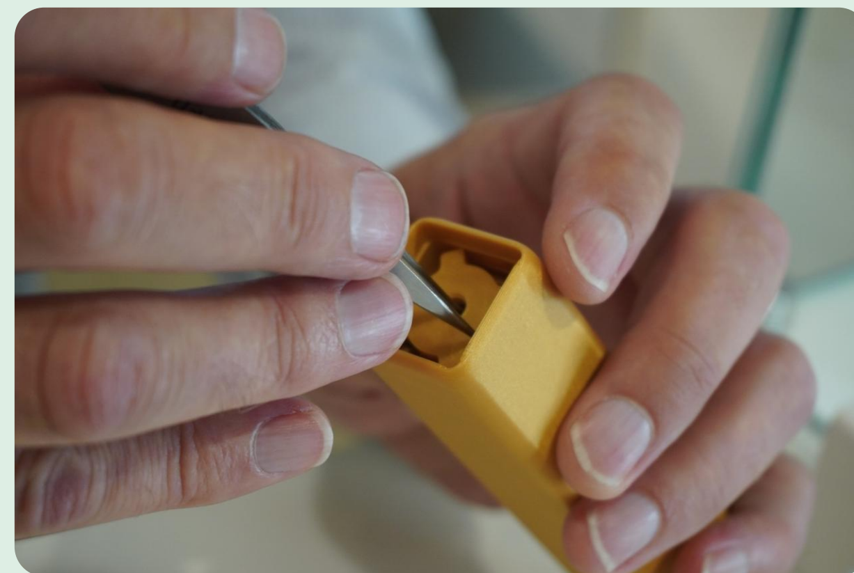
4 Releasing the retaining plate with tweezers. This is the step he misread, and a future iteration of the sheet should show the direction of rotation at steps two and three.
