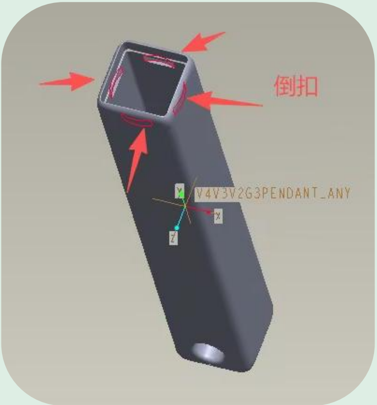
Figure 69. The retaining groove as the supplier saw it. 倒扣, the Chinese term for an undercut
