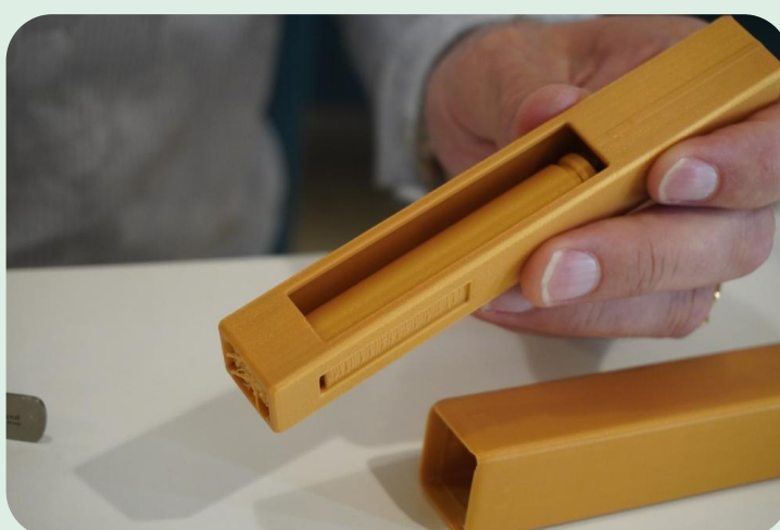
2 The cell in the inner assembly channel. A plastic spatula lifts it out. He does not stock one and was able to get it out with tweezers, so the kit now ships it.
