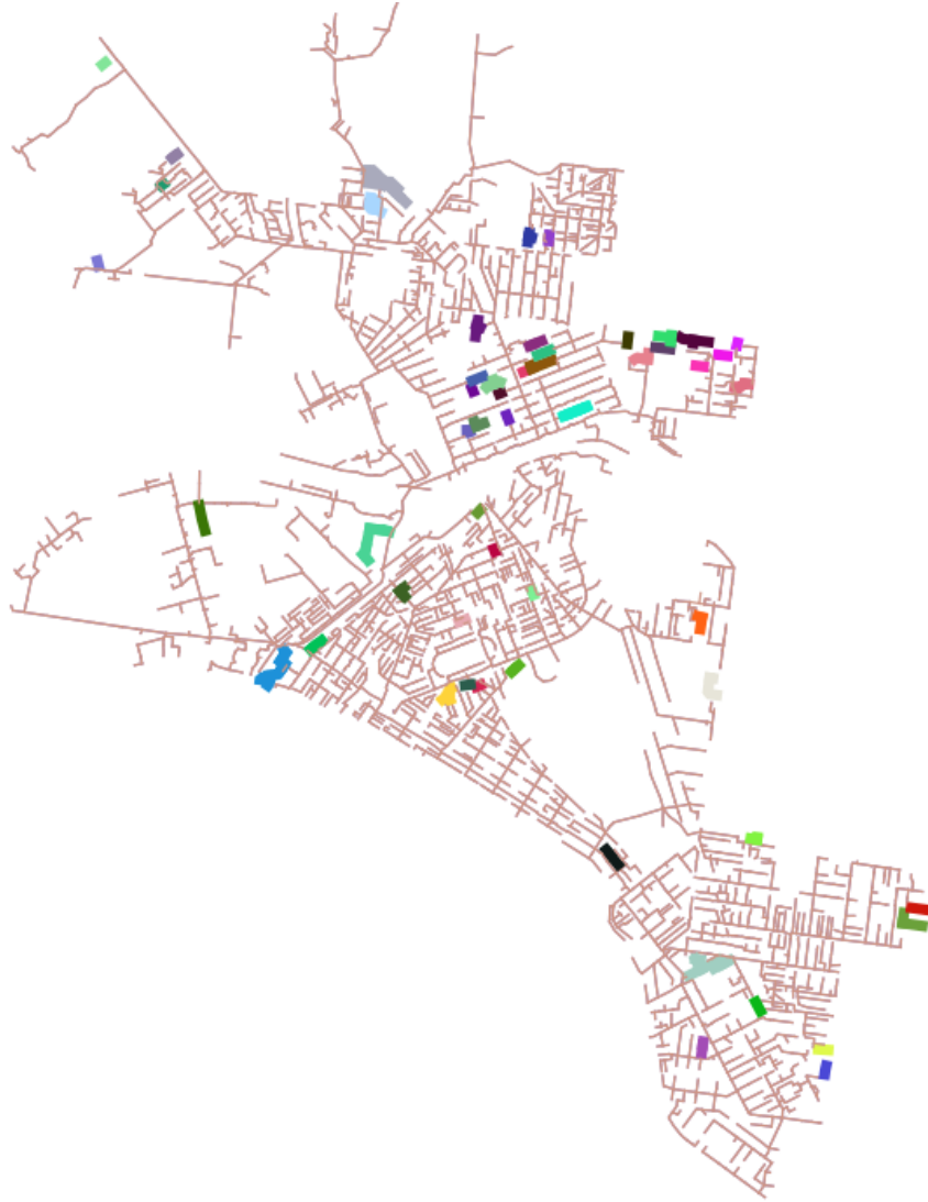
Figure 3.9: Disconnected components of the 57km 2 network. Disconnected components sub-graphs, defined as smaller graphs which are not joined to the main (larger) graph, are represented by coloured thick lines while the main network is shown with brown thin lines.
