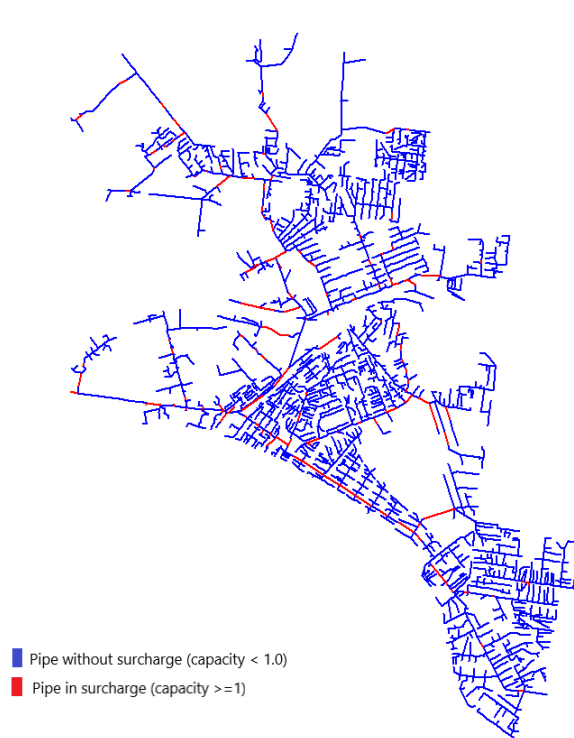
Figure 4.28: Real Network 57km 2 High Flow
