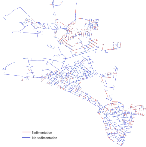
Figure 4.39: Real Network Sedimentation (57km 2 )
