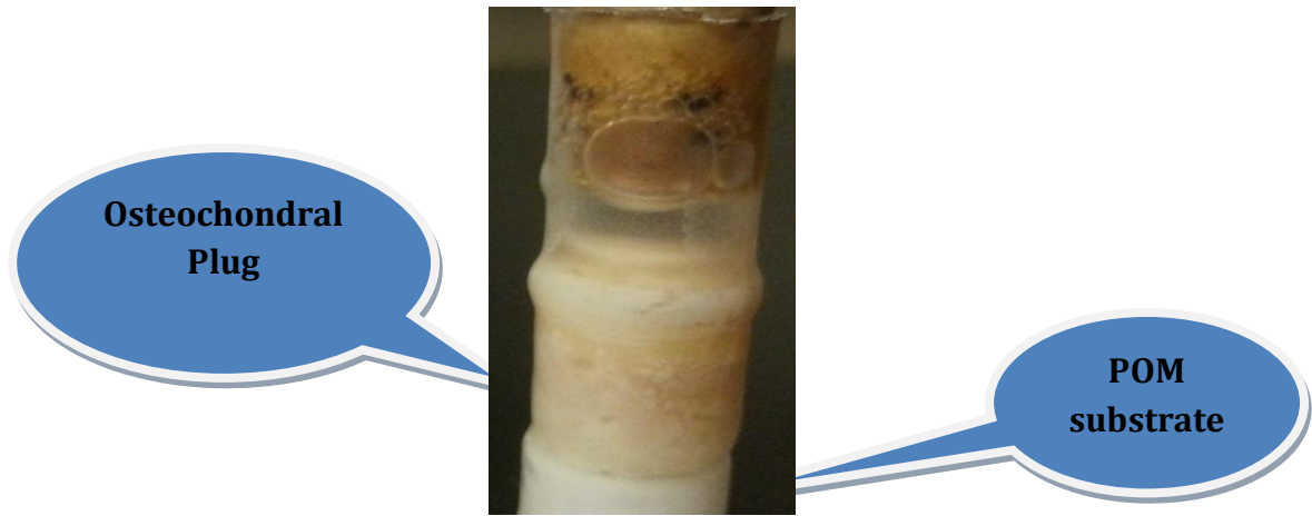
Figure 24: Representative Osteochondral plug with the associate POM substrate in order to achieve a total length of 15mm.
