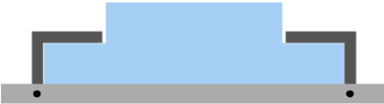
Figure SI3.6: The fabricated PDMS sample (blue) was placed on the force platform (light grey). A covering part from stainless steel (SS) with a squared void (dark grey) was placed on top of the sample to fixate it. Small magnets (black) were integrated in the force platform to fixate the SS covering part on the force platform.
