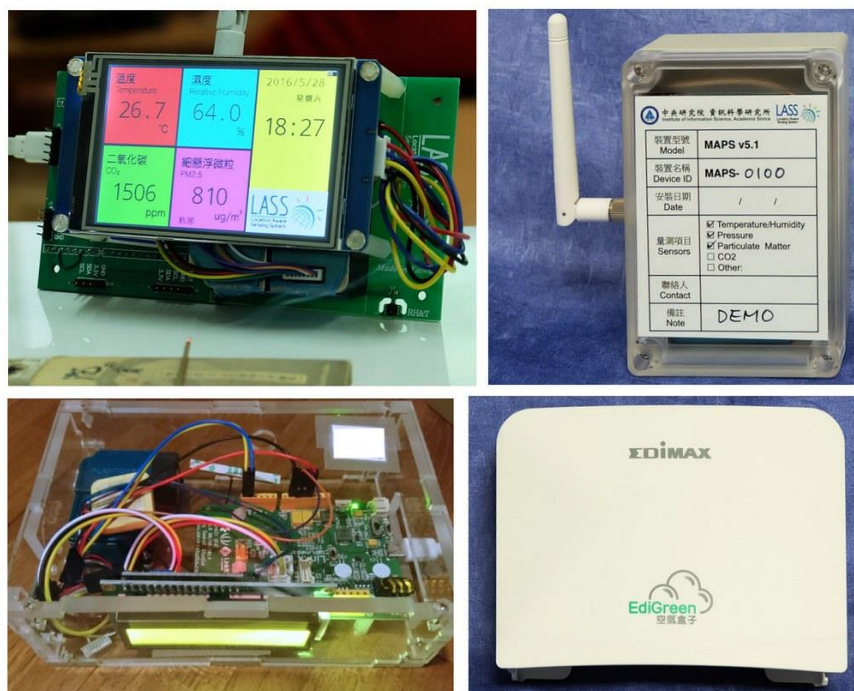
Figure 3-3. Different versions of AirBox in Taiwan. Original source: “Several common air quality micro-sensors with open data infrastructure and data upload feature: upper left and lower left: LASS AirBox; top right: MAPS by Academia Sinica; lower right: Edimax AirBox.” by Chen W.-Z. (2017), licensed under CC BY-NC-ND 3.0 TW.
