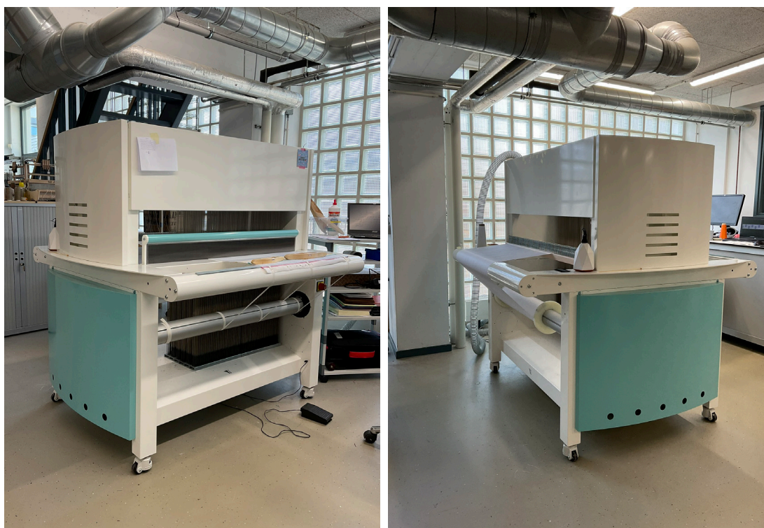
Figure 29: Materials Lab, TU Delft, Jacquard TC2 loom produced by Digital Weaving Norway
