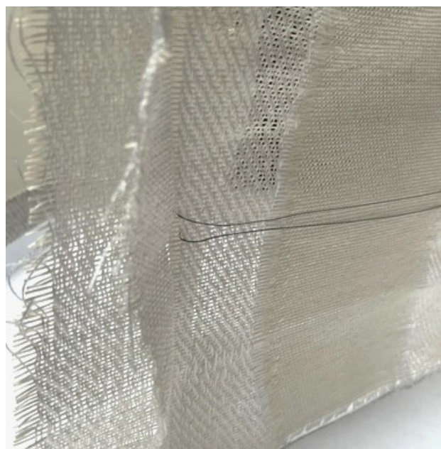
Figure 56: Close-up view of the SMA integration
