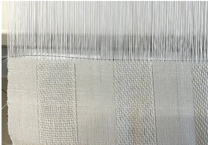
Figure 93: SMA integration during weaving
