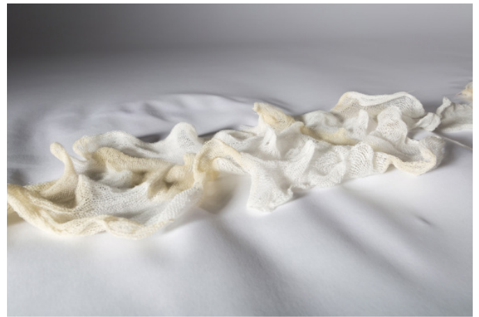
Figure 9: This fabric combines silk and linen with opposing orientation (twist direction) in combination with irregular patterns of stitch transfer to produce organic curls and folds when actuated. (Scott, 2015)
