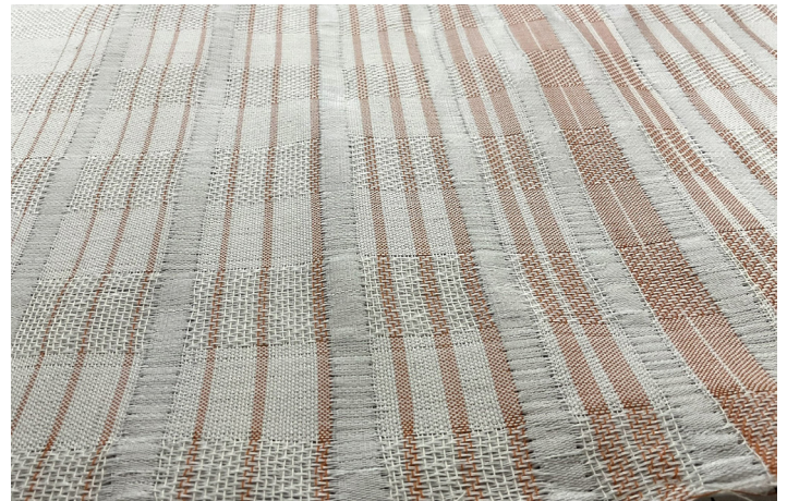
Figure 92: Front side- SMA is hidden
