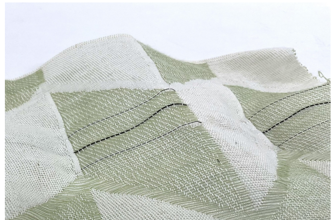
Figure 62: Close-up view on the SMA integration
