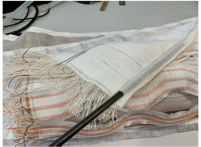
Figure 98: Metallic rod insertion in the double layered part for additional weight
