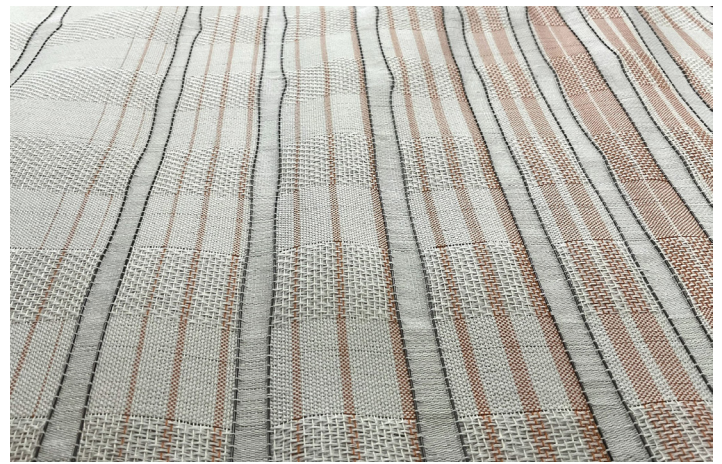
Figure 94: Back side- SMA is exposed
