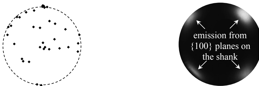
Fig. 5.45. The symmetry of the emission pattern is affected by the operating conditions. Left: the positions of the island remains on the facet with respect to the edge of the pattern (dashed circle) just before the series is finished, for all ring series recorded. Right: emission pattern for the emitter showing the emission from the {100} terraces on the shank.
