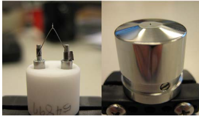
Fig. i.2. Schottky emitter with and without suppressor cap.
