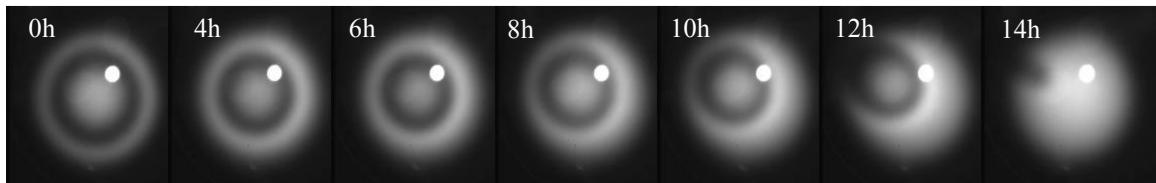
Fig. 5.46. Evolution of the emission pattern showing a change from symmetric to asymmetric. The patterns are recorded for an extraction voltage of 3.6 kV and a filament current of 2.36 A. The first pattern is taken right after applying these conditions.
