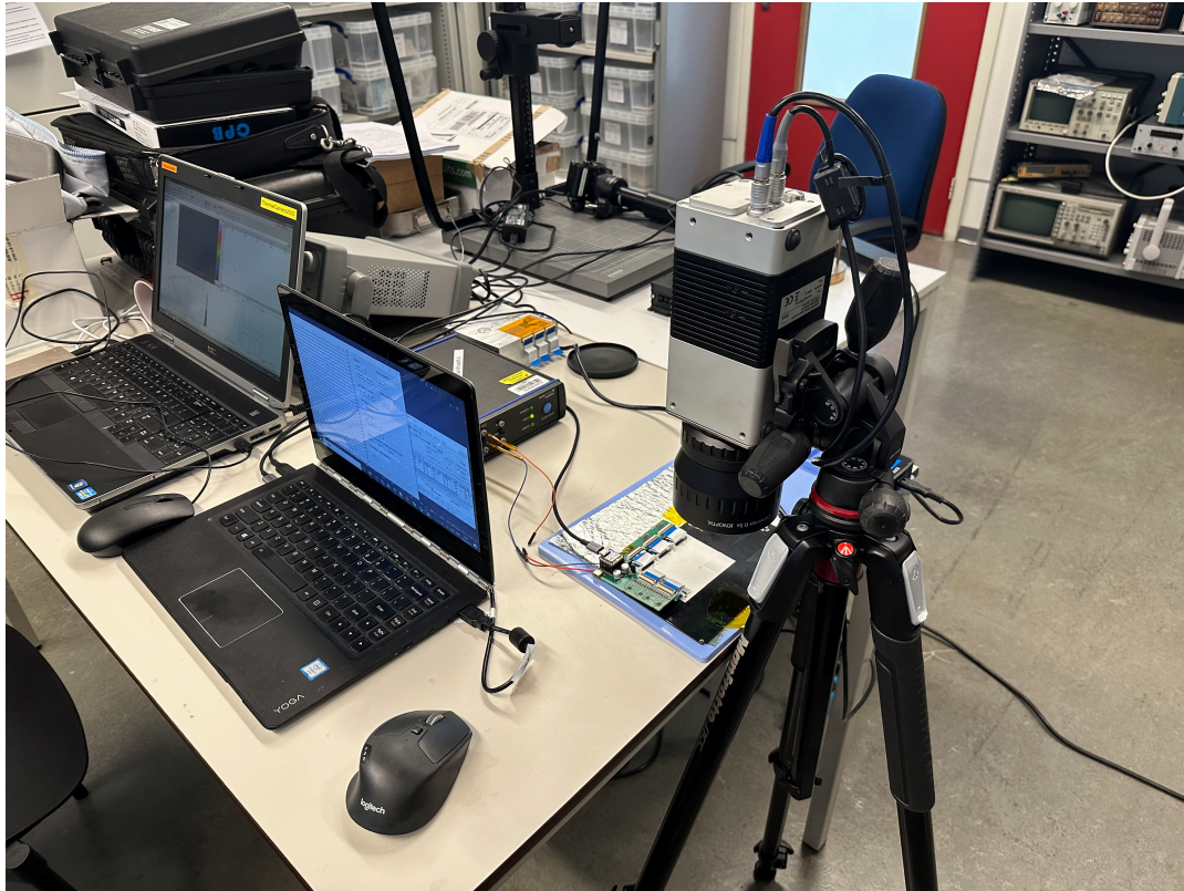
Figure 2.13: The thermal characterization experimental setup for 48x32 mini LED matrix with white substrate
