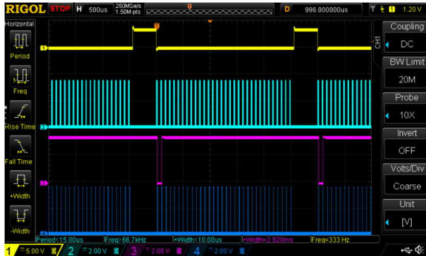
Figure 2.10: Scanning timing signal measured at GPIO0 (yellow), DCLK (light blue), RDAT (pink) and RCLK (Blue)
