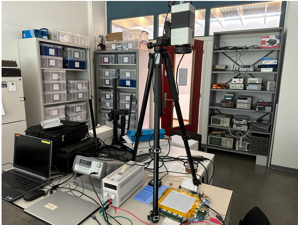
Figure 4.8: The experimental setup for thermal measurement of 160x160 mini LED matrix
