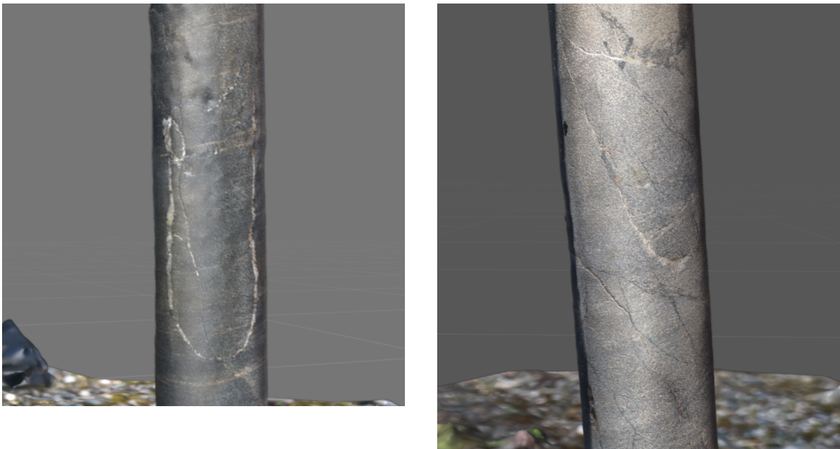
Figure A.4: Different types of fractures within the Buntsandstein in farfield stress.
