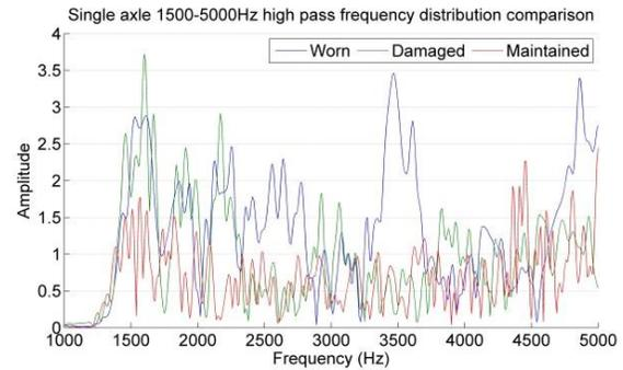
Figure 8 Vertical acceleration 1500-5000Hz high pass responses comparison
