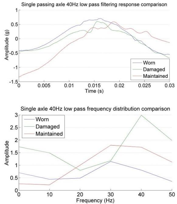
Figure 5 Vertical acceleration 40Hz low pass responses comparison (Time and frequency domain, same below)
