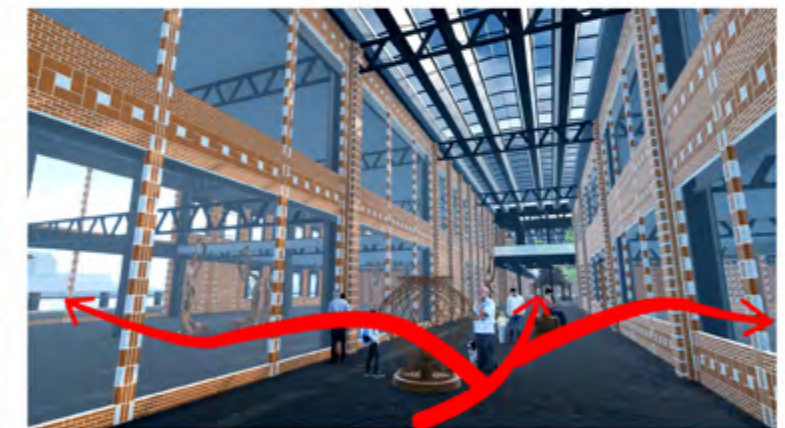
4 Wind enters the clusters sideways, providing clean air as it passes along the atrium
