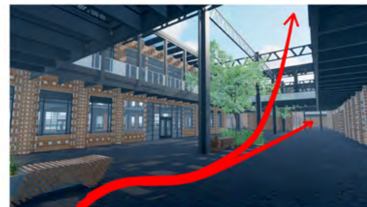
3 Open courtyard acts as green lung and buffer zone to normalise excess wind pressure
