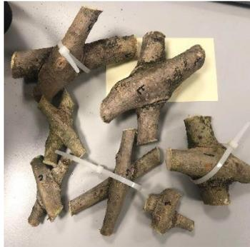
Figure 48. Crosswise connection specimens
