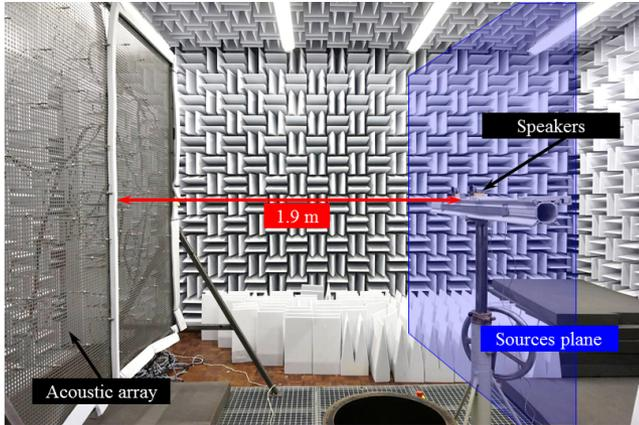
Figure 3.29: Experimental set-up in TU Delft V-tunnel
