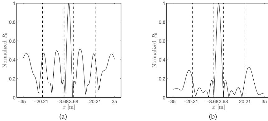
Figure 3.7: Comparison of two 2-D intersections of the beamforming images of Fig. 3.6 at  $y = 0\text{m}$  with corresponding value of  $J = 47.52$  for (a) and  $J = 8.48$  for (b). The normalized pressure amplitude is given on the vertical axis.
