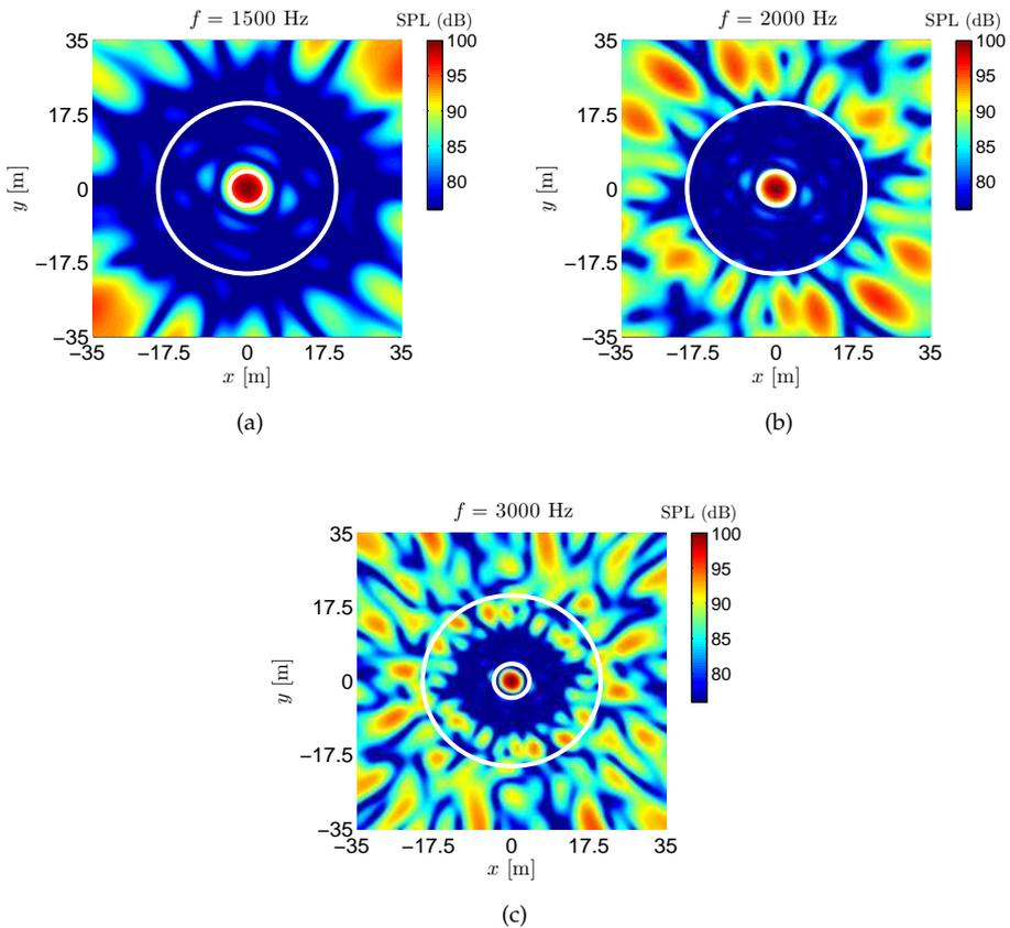
Figure 3.12: Beamforming with the microphone configuration given in Fig. 3.10d for a simulated source signal at the origin at frequency (a)  $f = 1500$  Hz, (b)  $f = 2000$  Hz and (c)  $f = 3000$  Hz.
