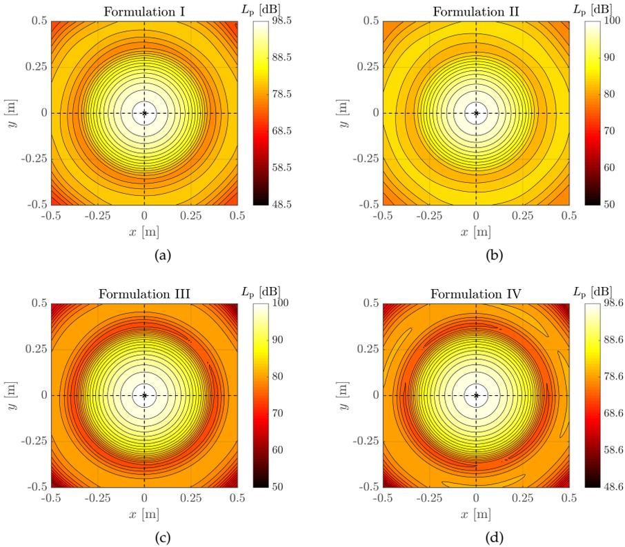
Figure 2.7: Comparison of beamforming results for the different steering formulations of the  $xy$  plane which is parallel to the planar microphone array.
