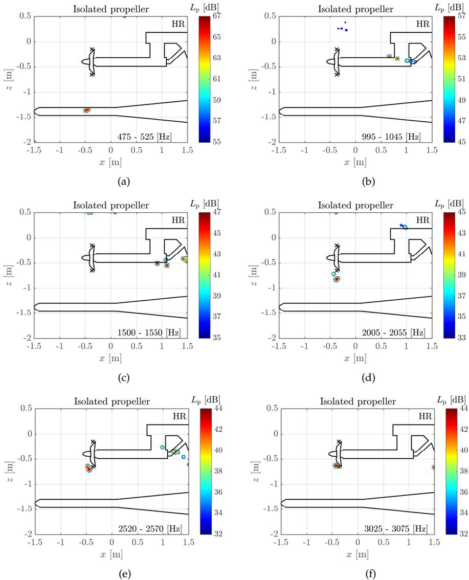
Figure 5.20: Narrowband adaptive HR-CLEAN-SC beamforming (HR) for the isolated propeller with frequencies listed in the subfigures.
