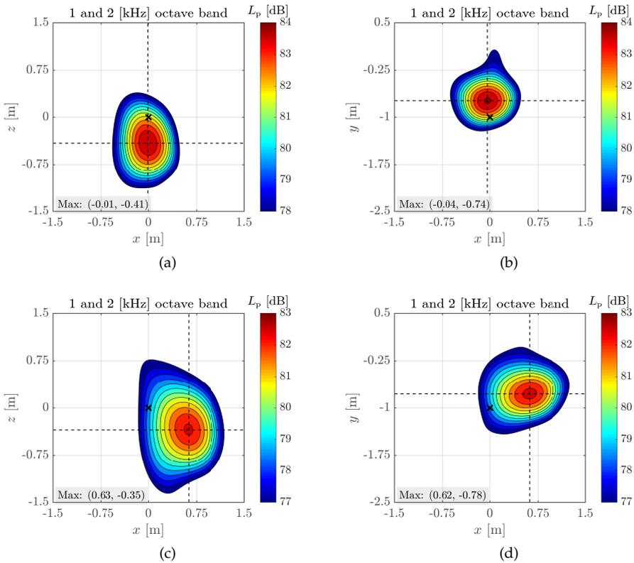
Figure 5.10: Beamforming for the loudspeaker over 1 and 2 kHz octave band, (a)  $xz$ -plane at  $y = -1.0$  m no flow, (b)  $xy$ -plane at  $z = 0$  m no flow, (c) and (d) have the addition of flow with  $U = 60$  m/s.
