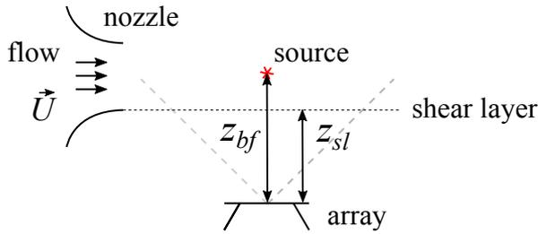
Figure 2.10: Schematic of the distances used for the simple shear layer correction. The correction provide good results for scan points within the dashed gray lines and  $M < 0.25$ .
