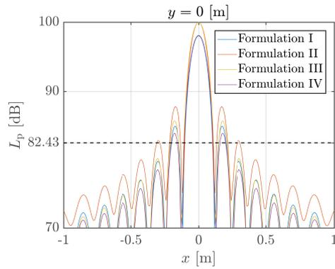
Figure B.4: Intersection of the microphone configurations given in Fig. B.1 (b) and the beamforming result  $y = 0$  m for four different steering vector formulations. The lowest attainable MSL is given by the dashed line.
