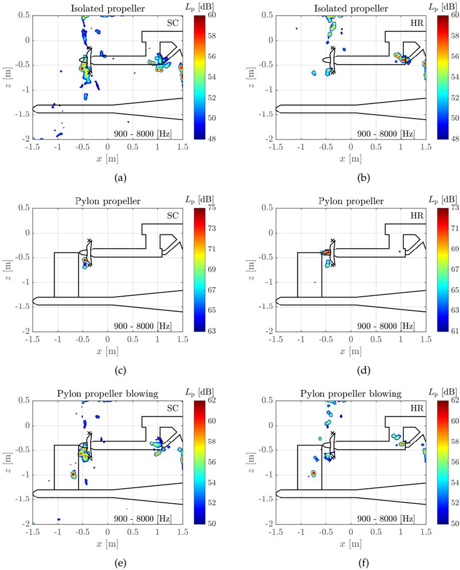
Figure 5.17: CLEAN-SC beamforming (SC) for (a), (c) and (e). Adaptive HR-CLEAN-SC (HR) for (b), (d) and (f). The three configurations isolated propeller, pylon propeller and pylon propeller with blowing can be seen arranged in the rows.
