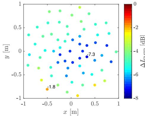
Figure 6.10: Difference in OSPL of the propeller at 7500 RPM, with incoming airflow, in the acoustic array when the duct is introduced (filtered between 50 to 8000 Hz). The outline of the duct on the array is shown in the center.
