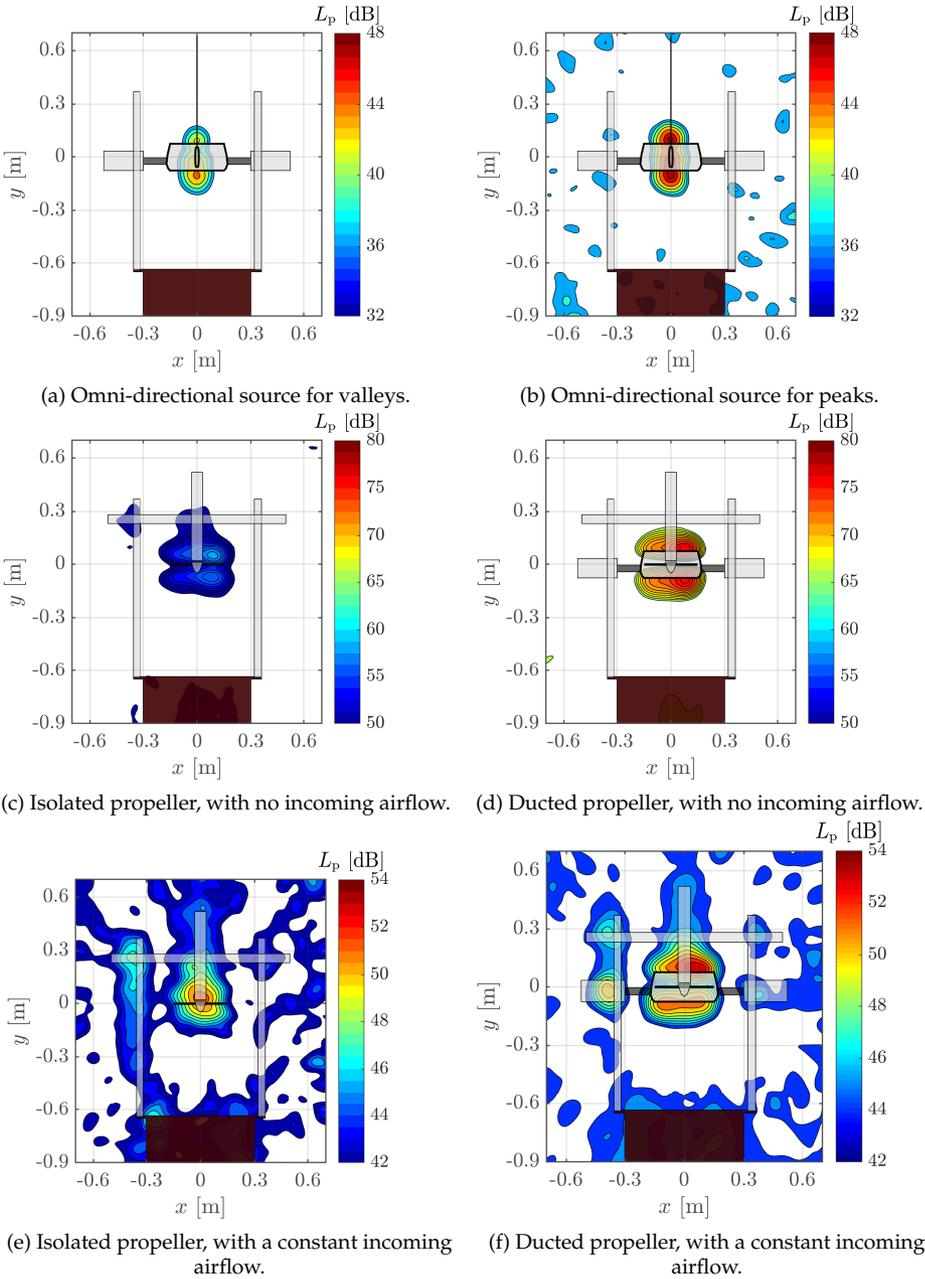
Figure 6.11: Beamforming of (a) and (b) are from the spectrum in Fig. 6.5 between 2 to 6 kHz. Beamforming of (c), (d), (e) and (f) are between 2 to 5 kHz.
