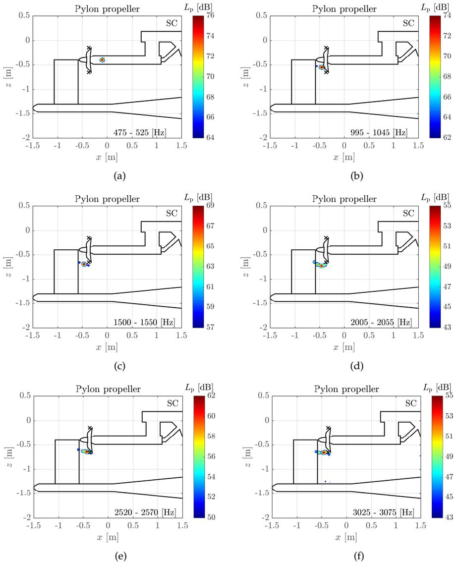
Figure 5.22: Narrowband CLEAN-SC (SC) for the installed pylon and propeller with frequencies listed in the subfigures. No pylon blowing is applied.
