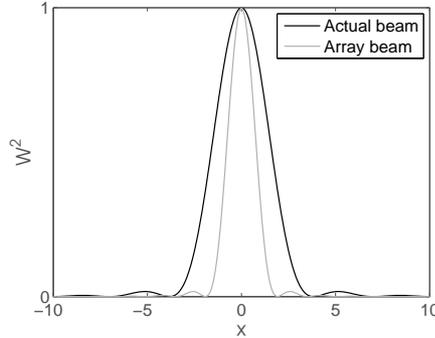
Figure 3.14: Cross-section of Fig. 3.3 through  $(0,0)$  of Airy pattern for the maximum array aperture (array beam) and aperture typically encountered during the optimization (actual beam). Actual beams are always larger or equal to the array beam.
