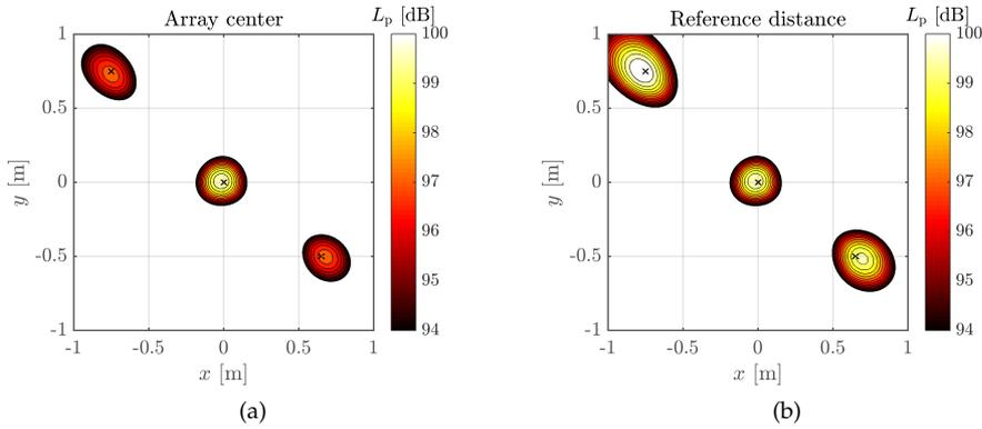
Figure 2.9: Comparison of beamforming when evaluating the source map to the array center (a) or to a constant reference distance  $R_0$  in (b). The source positions are given by the crosses and are simulated having the same SPL of 100 dB at  $R_0$ . In (a) the SPL differs as the distances of the array center to the outer sources are larger than to the source at the origin.
