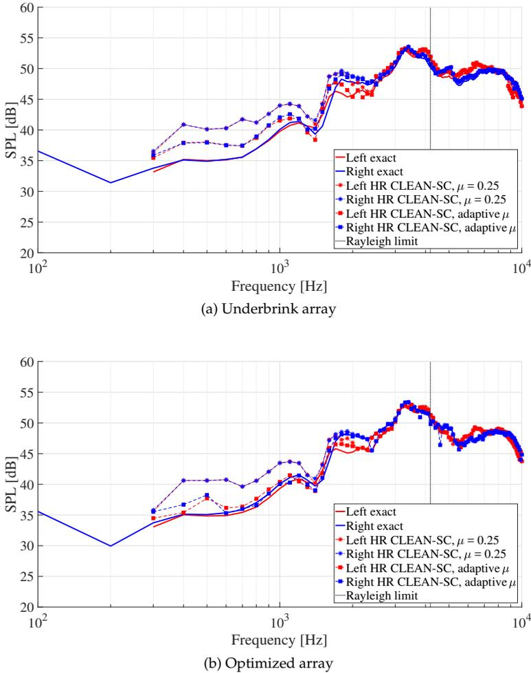
Figure 3.35: Resolved SPL of two sound sources with 10 cm separation versus beamforming frequency, obtained from HR CLEAN-SC beamforming of experimental data with a constant and adaptive  $\mu$ , compared with the exact SPL values
