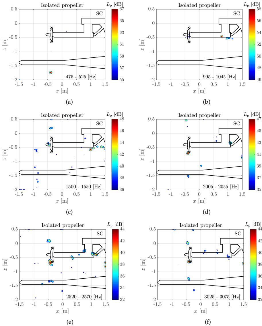
Figure 5.19: Narrowband CLEAN-SC beamforming (SC) for the isolated propeller with frequencies listed in the subfigures.
