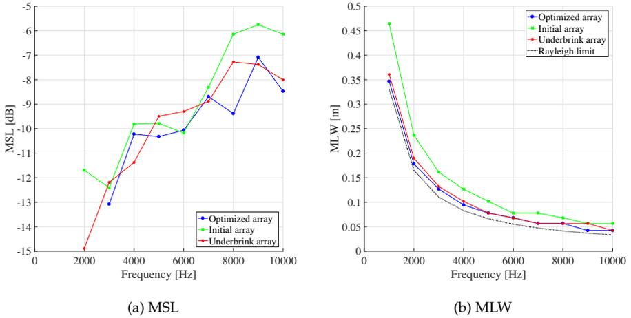
Figure 3.22: MSL and MLW of the optimized array obtained from simulations compared with those from the initial and the Underbrink arrays
