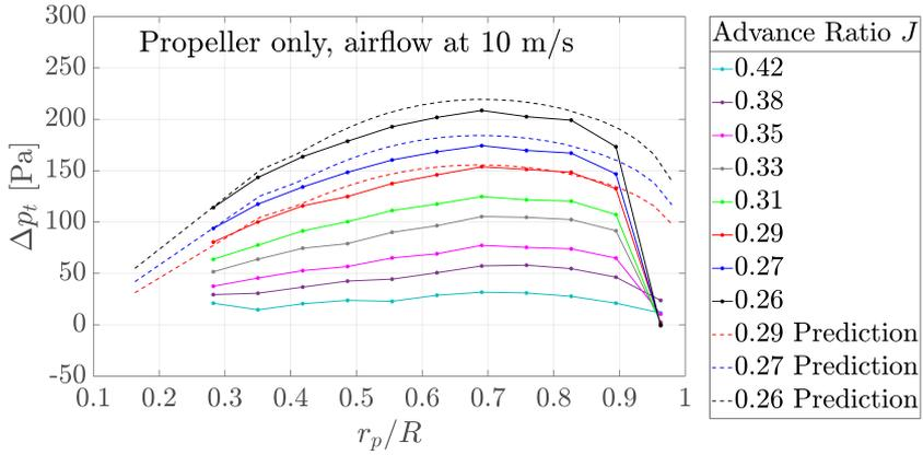
Figure D.1: Difference over the blade span between the total pressure above the propeller disk and the free stream total pressure,  $\Delta p_t$ . Solid lines are determined from experiment and dotted lines from the BEM model.
