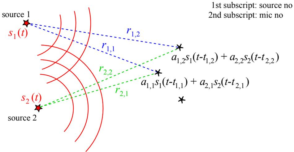
Figure 2.3: Depiction of two sources,  $s_1$  and  $s_2$ , and the corresponding expressions for the received signals at the microphones. For a single microphone the contribution of both sources needs to be taken into account.
