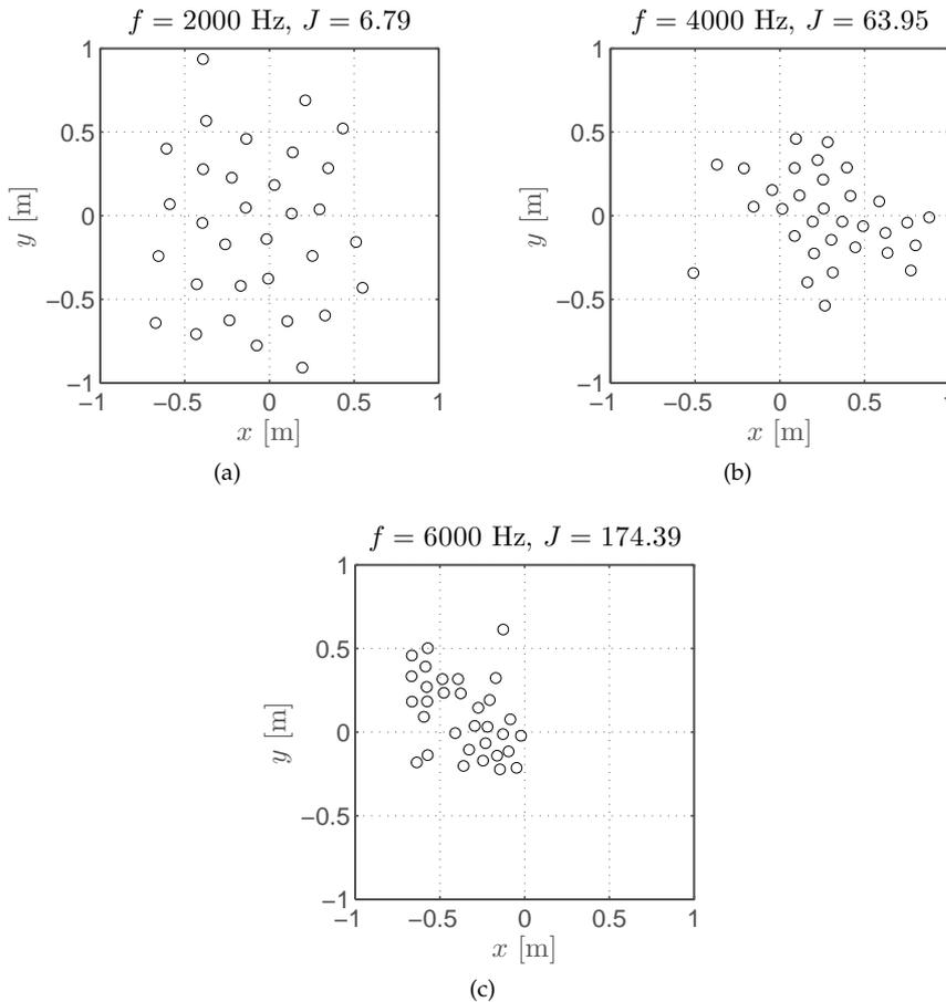
Figure 3.13: Microphone configurations after optimization for frequencies (a)  $f = 2000$  Hz, (b)  $f = 4000$  Hz and (c)  $f = 6000$  Hz.
