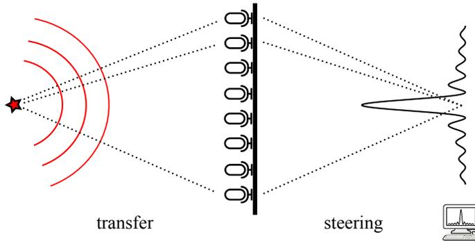
Figure 2.5: A conceptual microphone array with a single source on the left side where the *transfer* of the signal takes place to the microphones. On the right side the post-processing part is done with a computer using the *steering* of the acquired microphone signals. Ideally, the transfer- and steering-functions are inverse functions of each other.
