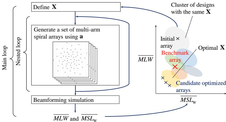
Figure 3.19: Schematic diagram of the optimization method used
