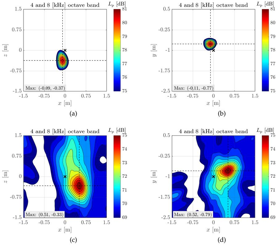
Figure 5.11: Beamforming for the loudspeaker over 4 and 8 kHz octave band, (a)  $xz$ -plane at  $y = -1.0$  m no flow, (b)  $xy$ -plane at  $z = 0$  m no flow, (c) and (d) have the addition of flow with  $U = 60$  m/s.
