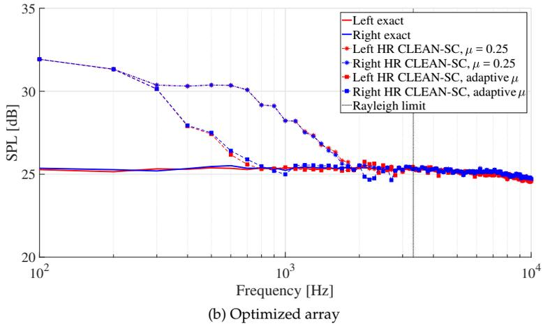
Figure 3.26: Resolved SPL of two closely-spaced sound sources versus beamforming frequency, obtained from HR CLEAN-SC beamforming simulations with a constant and adaptive  $\mu$ , compared with the exact SPL values
