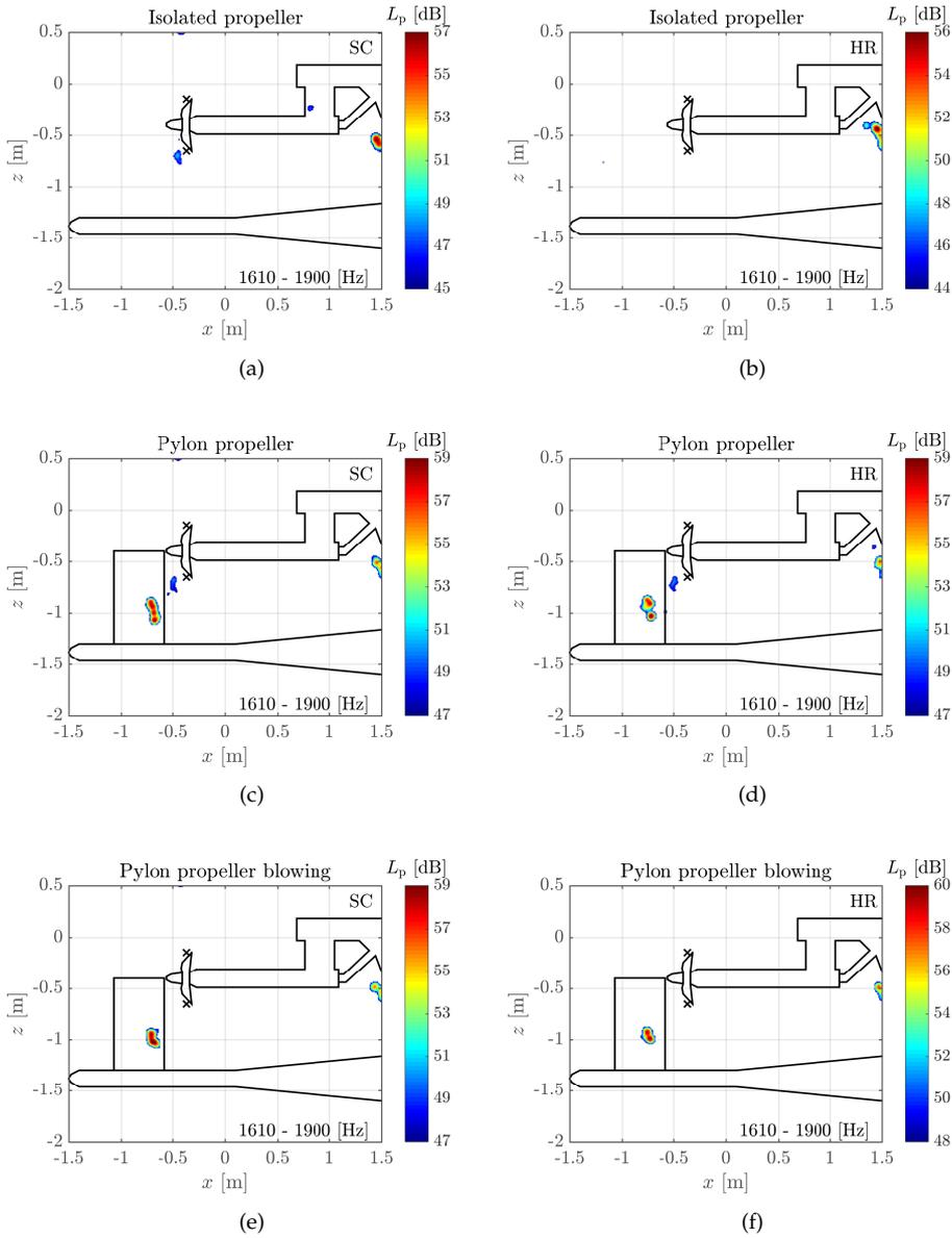
Figure C.4: CLEAN-SC (SC) and adaptive HR-CLEAN-SC (HR) for 1610 to 1900 Hz for the three configurations.
