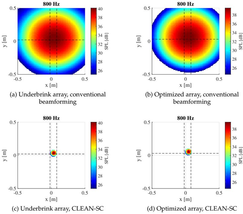
Figure 3.36: Source maps of two closely-spaced sources for various beamforming (CB and CLEAN-SC) algorithms at 800 Hz, using experimental data
