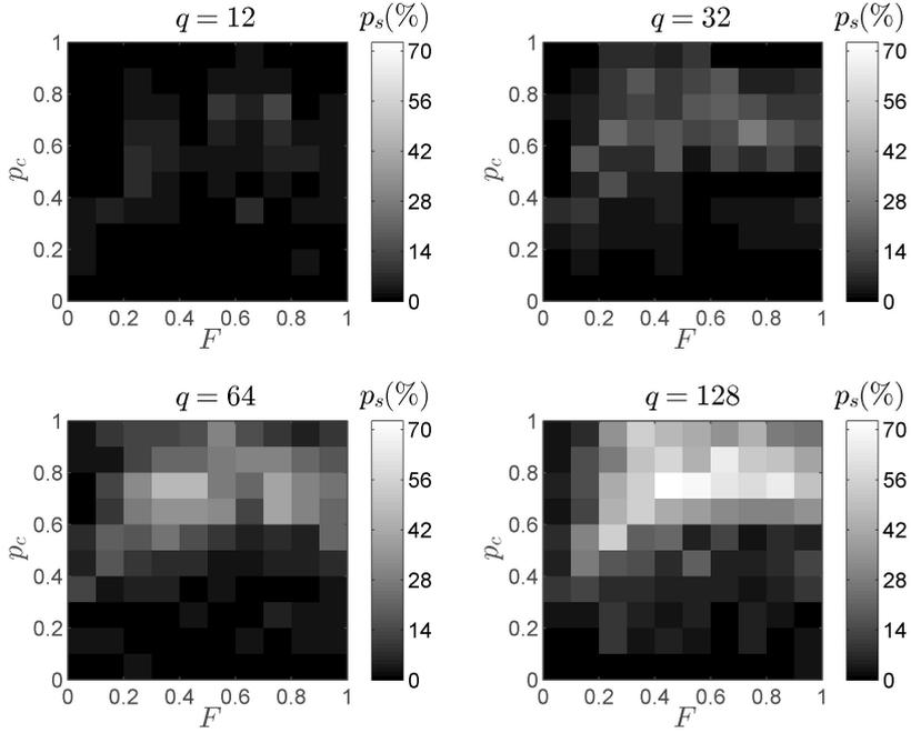
Figure 4.3:  $p_s$  as a function of  $p_c$  and  $F$  for four different population sizes  $q = 12, 32, 64$  and  $128$  with  $N_G = 600$  using the highest frequency,  $f = 6000$  Hz, for the Bartlett energy function.
