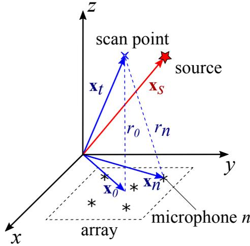
Figure 2.6: Schematic for the vectors and distances used in this section for an array of 5 microphones on the  $xy$ -plane. As an example this case has the scan point  $\vec{x}_t$  not matching the source position at  $\vec{x}_s$ .
