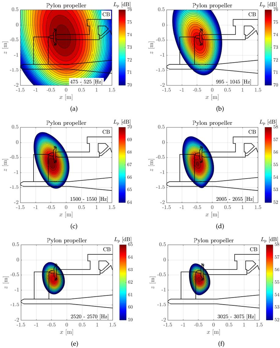
Figure 5.21: Narrowband conventional beamforming (CB) for the installed pylon and propeller with frequencies listed in the subfigures. No pylon blowing is applied.
