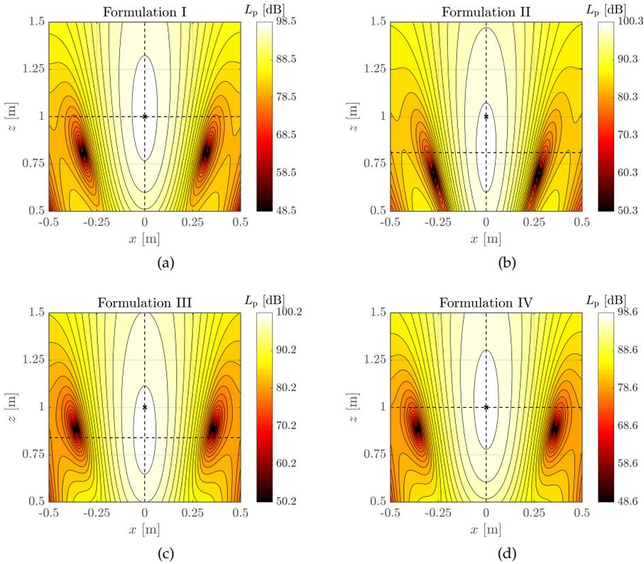
Figure 2.8: Comparison of beamforming of the different steering formulations of the  $xz$  plane which is perpendicular to the planar microphone array.
