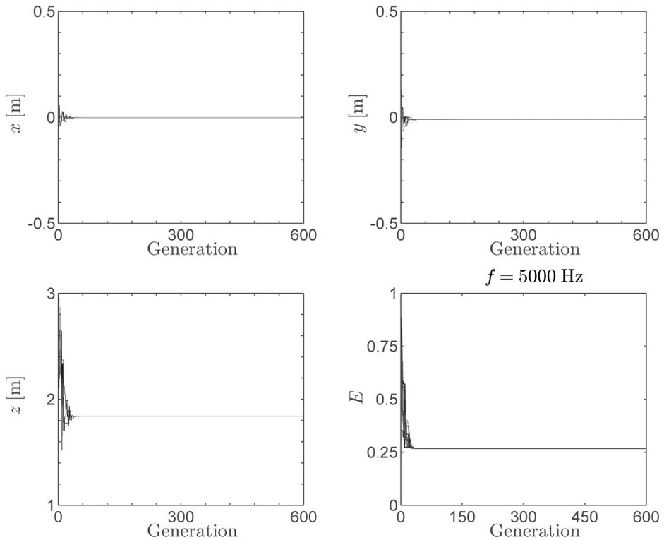
Figure 4.20: Convergence of the spatial coordinates ( $x$ ,  $y$ ,  $z$ ) belonging to three runs for the optimal setting of  $F = 0.4$ ,  $p_c = 0.75$  at the population size of  $q = 128$  and the case with the speaker emitting at 5000 Hz. In the last figure the energy ( $E$ ) is given as a function of generation for 10 independent runs.
