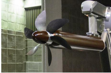
Figure 5.2: The six bladed propeller.
