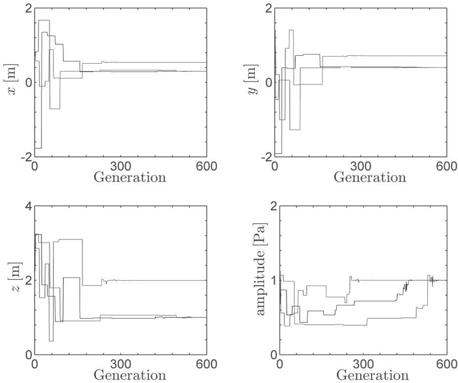
Figure 4.8: Convergence of the spatial coordinates  $(x, y, z)$  and source amplitude belonging to three runs for the optimal setting of  $F = 0.35$ ,  $p_c = 0.75$  at the population size of  $q = 128$ .
