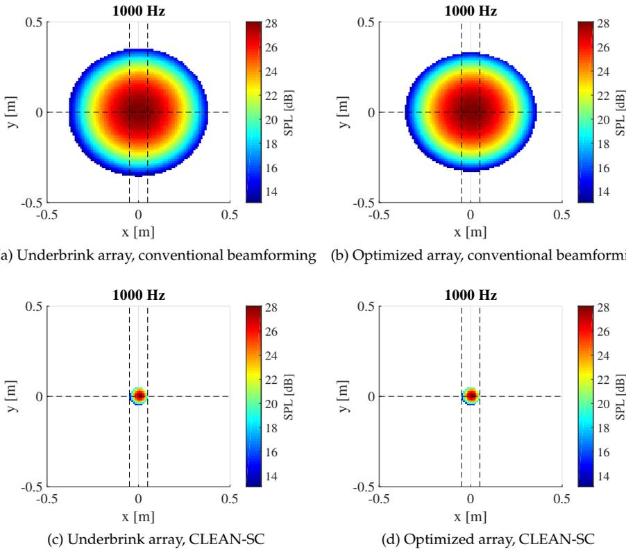
Figure 3.27: Source maps of two closely-spaced sources for various beamforming algorithms (CB and CLEAN-SC) at 1 kHz, using synthetic data
