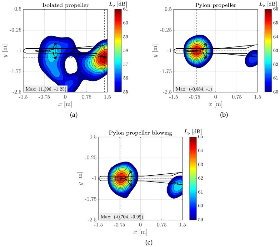
Figure C.5: Conventional beamforming (CB) in the  $xy$  plane at  $z = -0.97$  m for the three configurations (a) isolated propeller, (b) pylon propeller and (c) pylon propeller with blowing. The configuration and support can be seen to be outlined. The crosses indicate the two ends of the propeller plane.
