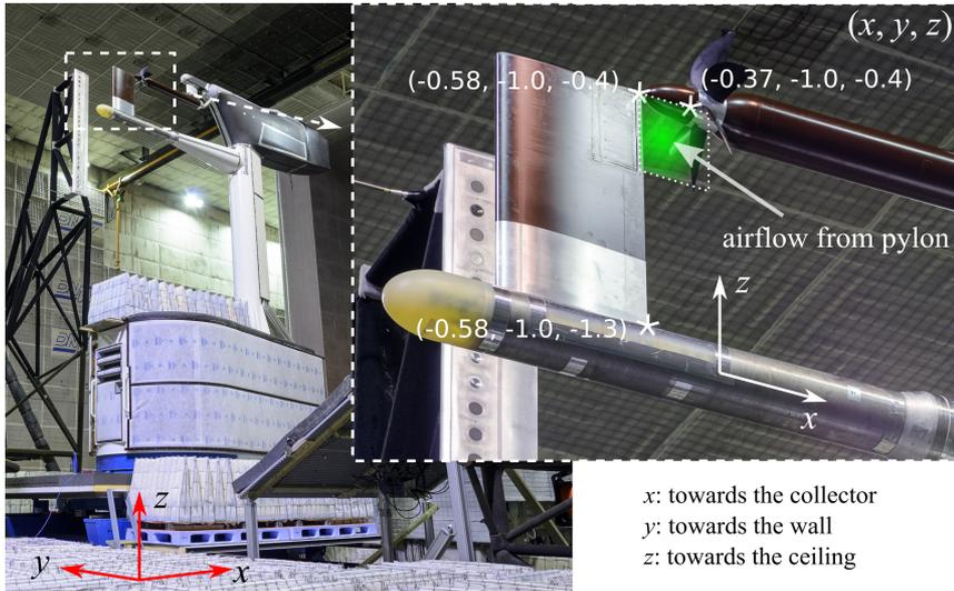
Figure 5.4: The installed pylon propeller configuration, with on the right a zoom-in. The coordinate system used can be seen together with three reference points.
