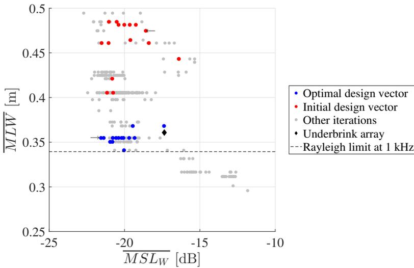
Figure 3.20:  $\overline{MLW}$  and  $\overline{MSL}_W$  of all array configurations considered in the optimization including the benchmarking Underbrink array, the arrows show the selected initial and optimal arrays
