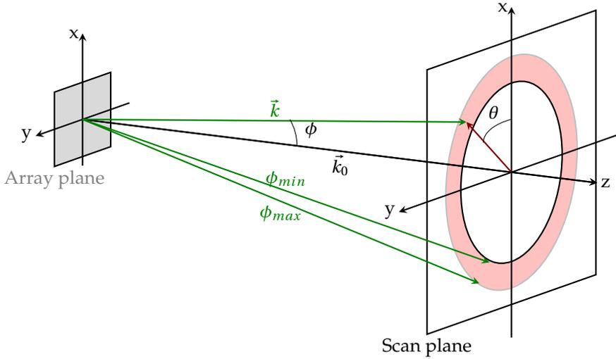
Figure 3.2: Relation between the wavevector  $\vec{k}$ , polar angle  $\phi$  and azimuthal angle  $\theta$ . The area of integration is shown in red. In practice the inner radius will be much closer to the origin.
