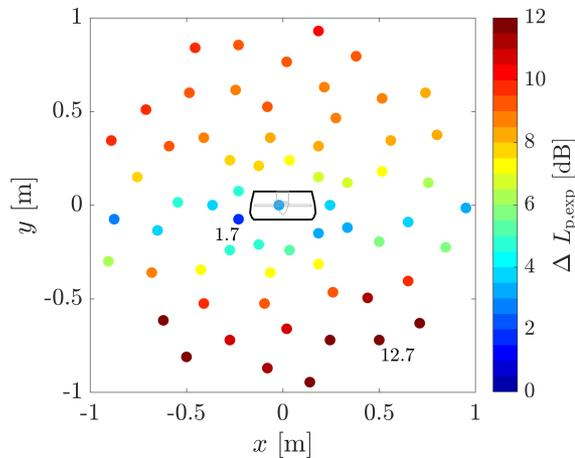
Figure 6.8: Difference in OSPL for the propeller at 7500 RPM, with no incoming airflow, in the acoustic array when the duct is introduced (filtered between 50 to 8000 Hz). The outline of the duct on the array is shown in the center.
