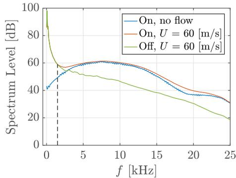
Figure 5.12: The spectrum levels of the Onera sparker source. The blue line indicates the source with no flow, red line with flow and green line flow but the sparker off. The speed of the wind is 60 m/s
