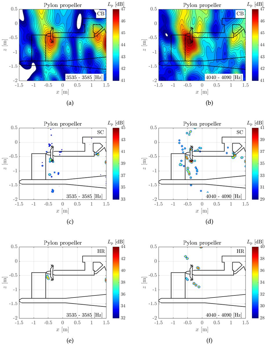
Figure C.2: Narrowband beamforming for the installed pylon and propeller with frequencies listed in the subfigures. Conventional beamforming (CB) in (a) and (b); CLEAN-SC in (c) and (d); and adaptive HR-CLEAN-SC in (e) and (f).
