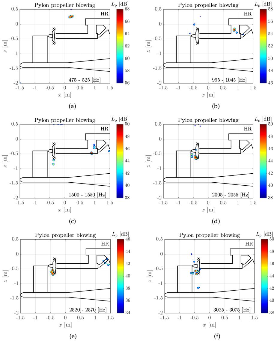
Figure 5.26: Narrowband adaptive HR-CLEAN-SC (HR) for the installed pylon and propeller with frequencies listed in the subfigures. Blowing is applied with a mass rate of 60 g/s.
