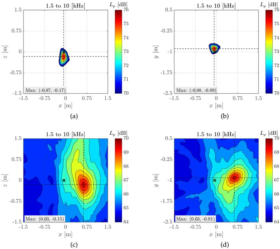
Figure 5.13: Beamforming for the Onera sparker source from 1.5 to 10 kHz, (a)  $xz$ -plane at  $y = -1.0$  m no flow, (b)  $xy$ -plane at  $z = 0$  m no flow, (c) and (d) have the addition of flow with  $U = 60$  m/s.
