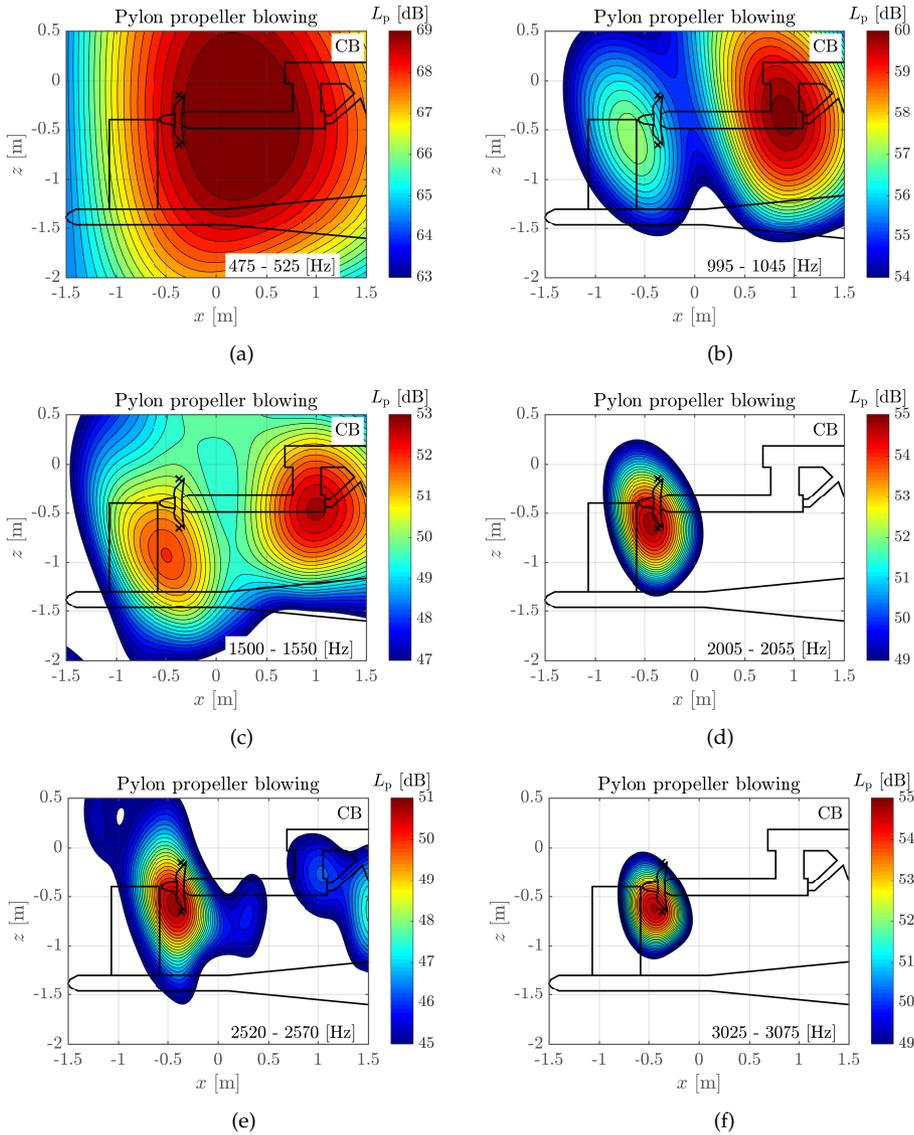
Figure 5.24: Narrowband conventional beamforming (CB) for the installed pylon and propeller with frequencies listed in the subfigures. Blowing is applied with a mass rate of 60 g/s.
