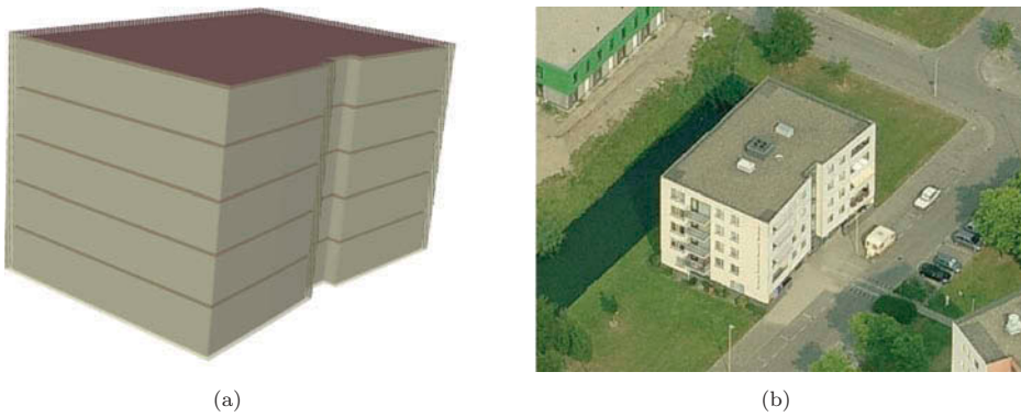
Figure 12. Comparison between: (a) a generated LOD2+ model and (b) the building from an aerial image taken from Bing Maps.
