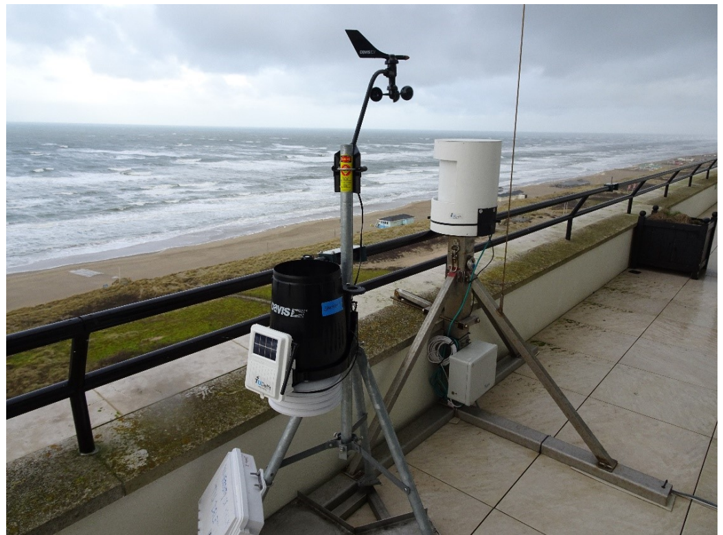
Figure 7. TLS and weather station installed on the upper balcony of the Huis ter Duin Hotel, Noordwijk, The Netherlands.
