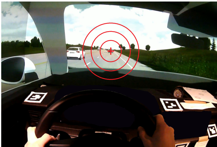
Figure 3.1: Illustration of the derivation of the light intensity, with the gaze marker depicted as a red cross, surrounded by rings in which each pixel has an equal contribution to the light intensity of that ring
