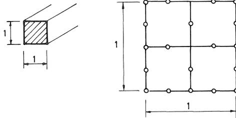
Fig. 6. Finite element mesh for the cross-section.
