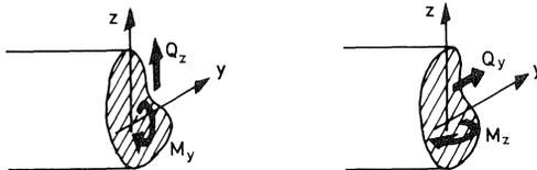
Fig. 4. Shear forces and bending moments.
