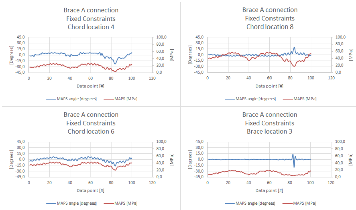
Figure 5.4: Principal stress angle changes and MAPS of Brace A connection, fixed constraints
