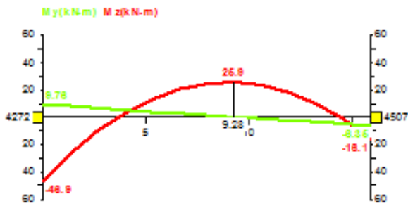
Figure 3.13: Brace A: Bending Moments due to Buoyancy
