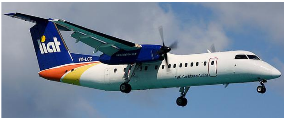
Figure 1.2: An aircraft just before landing. The flaps are deflected to increase the maximum lift coefficient.
