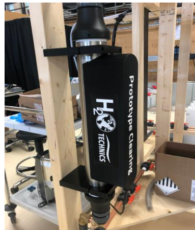
Figure 2. Ultrasound disinfection device provided by H2O TECHNICS
