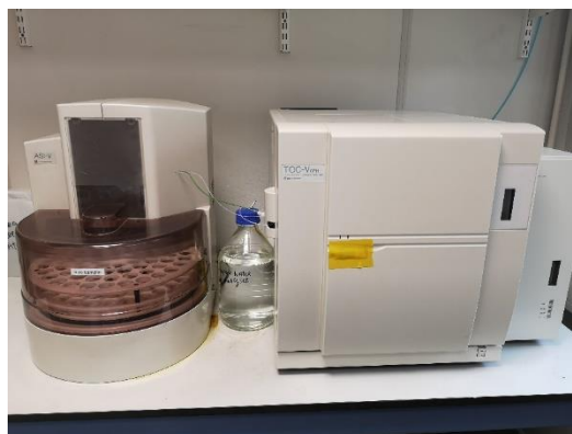
Figure 5. Shimadzu Total Organic Carbon Analyzer (TOC-VCPH)
