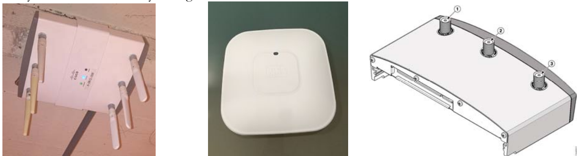
Figure 20: Picture of a TU Delft AP Installed at Architecture (a) and one at EWI (b). C: A radio Module that can be attached to the Core Body of the AP, to modify its Behaviour and Characteristics. Reproduced from Cisco (2013).
