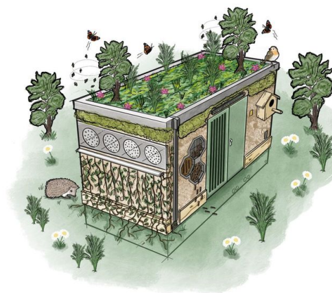
Figure 2.8: An example of the maximum level of nature inclusivity on the scale of nature inclusiveness for small utility buildings of Naturalis and KPN, featuring an intensive green roof, green facades, and other assets designed to support local wildlife (source: (Naturalis, 2022)).
