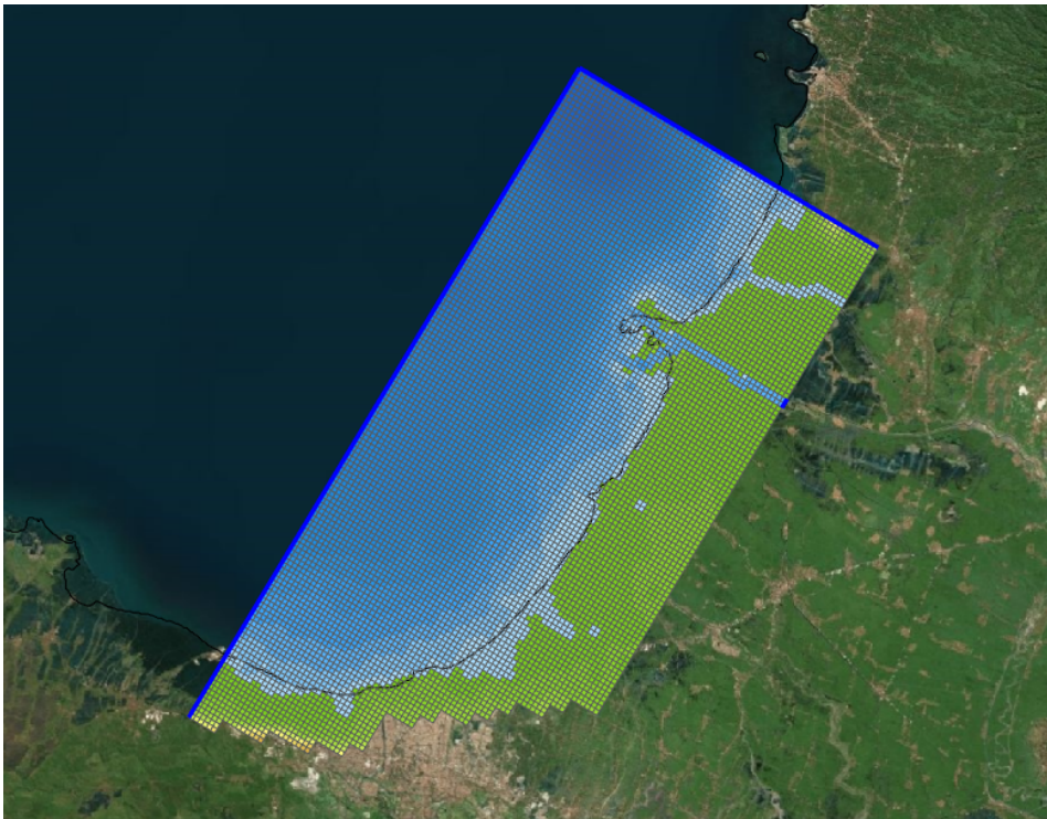
Figure 4.2: Model domain from Semarang city to the Wulan river, including the computational grid with cells of 333 by 333 m.
