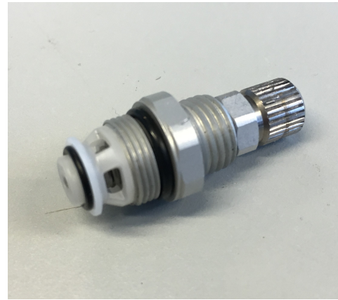
(b) Photo of the core of the Festo QS-4 restrictor. It should be installed into the pneumatic actuator to reduce the internal volume
