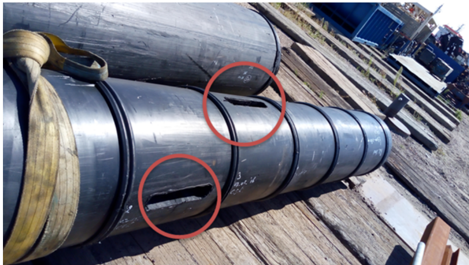
Figure 1.4: Custom made pipe section with slots of length comparable to the inner diameter of the pipe and width comparable to the pipe wall thickness. Slots are circled in red. Picture taken by author in the yard of a Dutch HDD contractor.
