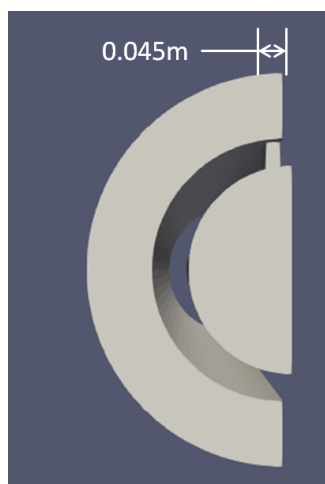
Figure 4.3: Side view of the geometry. Note the dimensions of half-slot width. Use of symmetry is made for this case to save up on computational time.
