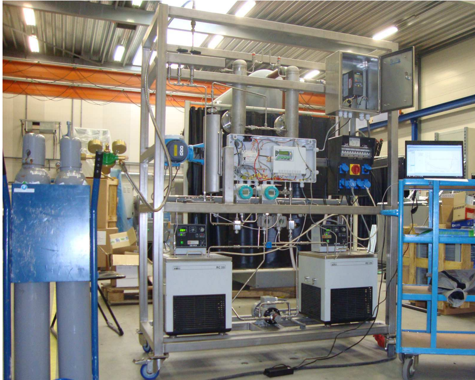
Figure 4-1: Photograph of the developed experimental CO_2 hydrate production set-up.
