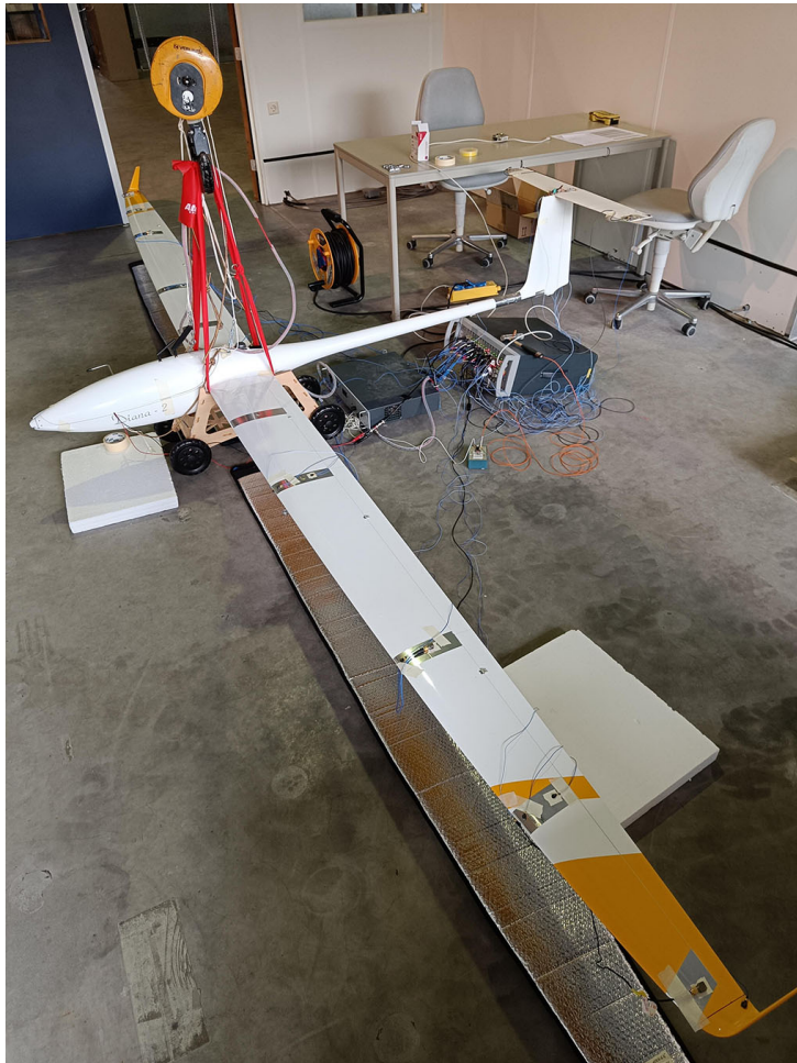
Figure 3.6: Ground vibration testing setup.
