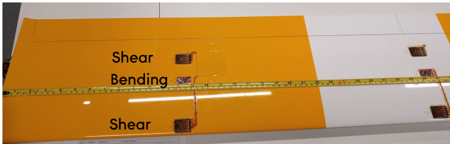
Figure 3.4: Strain gauge placement on the wings.
