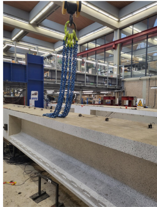
Figure 3.2: (left) Cross-section of the girder and (right) chain dragging on top of the girder [9].
