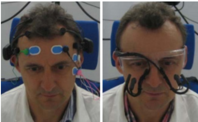
Figure [32]: Subject equipped with EMG, EEG and ECG (left) and with an eye tracker ECG (right) (Iodice, 2018)
