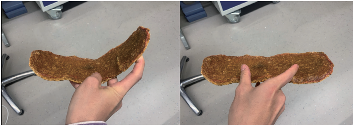
Figure 62. Mandarin composite for sole part of shoes shows its flexibility
