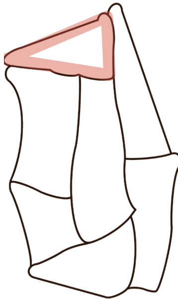
Figure 91. The rim part becomes brittle leading the decrease of tensile strength
