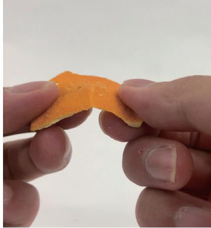
Figure 52. An orange peel became flexible after sanding the mesocarp part
