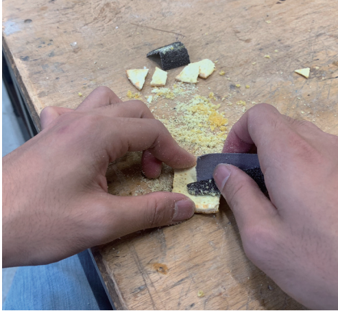
Figure 51. Removing the mesocarp part of orange peel with sand paper
