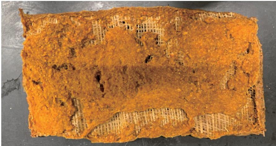
Figure 63. Uneven thickness of mandarin pulp after adding banana fiber structure
