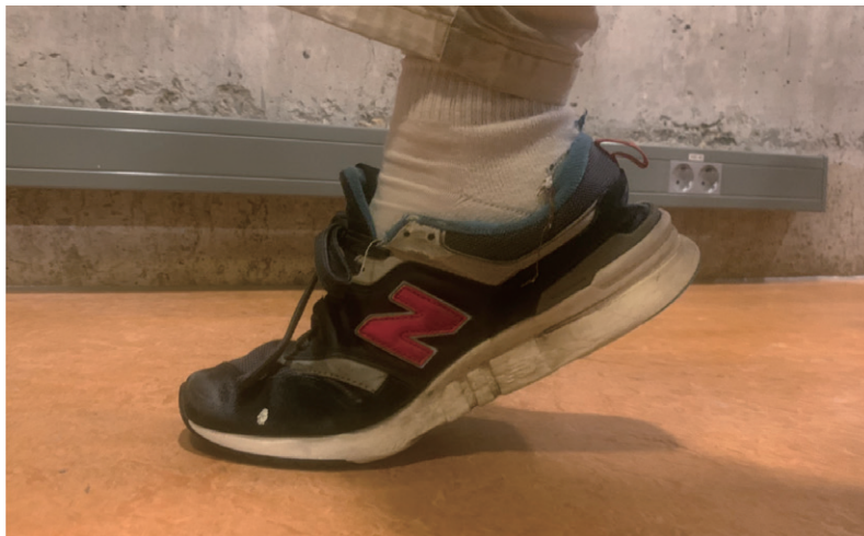
Figure 26. New Balance sneaker exhibited deformation in the forefoot region
