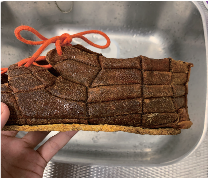
Figure 116. The shoes showed the water-repellent ability
