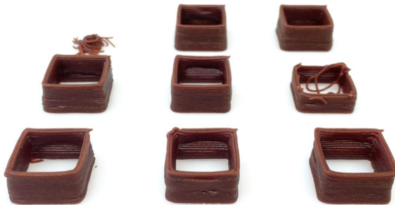
Figure 10. Nozzle clogging resulting in under-extrusion (left) or complete blockage (right)
