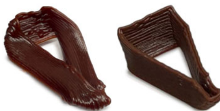
Figure 9. Impact of airflow on print quality
