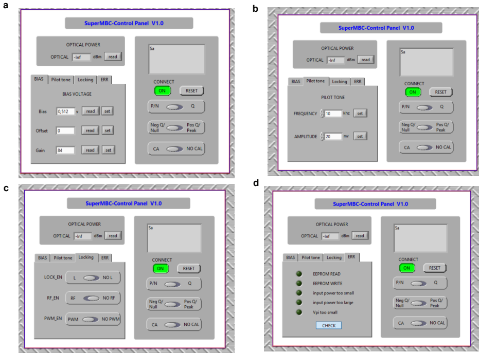
Figure 3.3: MBC-SUPER board settings on GUI when used in " Quad^+ / Quad^- " mode. The board works with a photodiode that receives part of the light signal from the EOM modulator, and adjusts the bias voltage on the EOM so that the EOM works at 50% transmission point with linear amplitude modulation.
