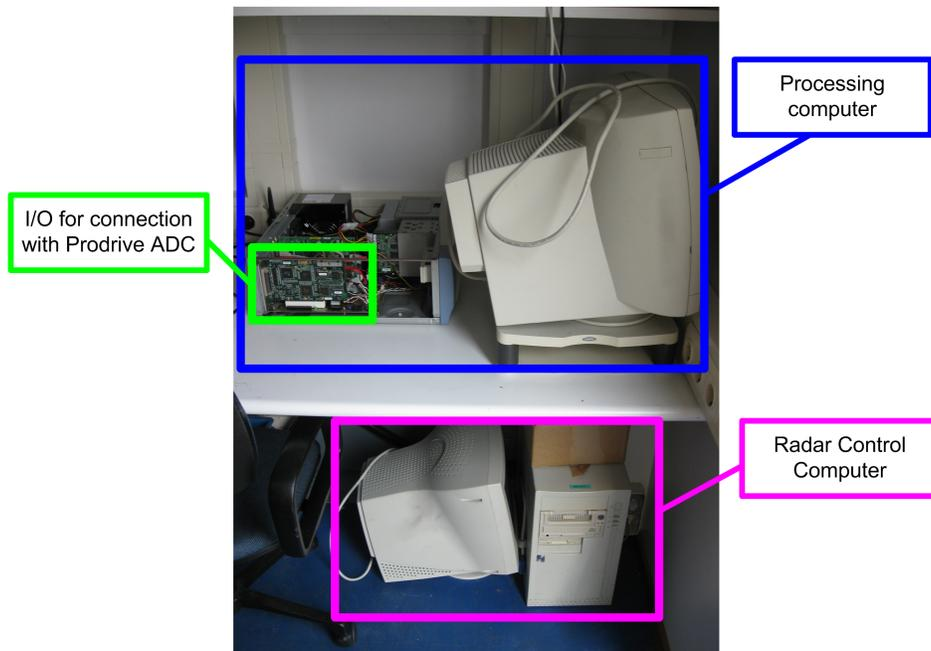
Figure E.5: Current Hardware Configuration
