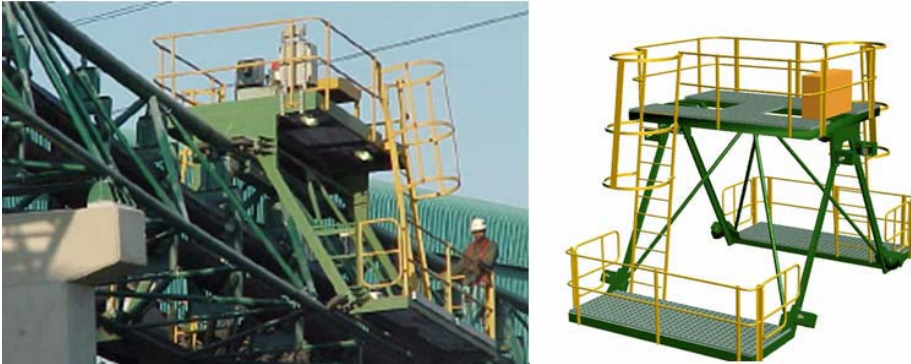
Figure 6.1: Maintenance trolley installed on the Richards Bay Coal Terminal, Republic of South Africa (courtesy CKIT).
