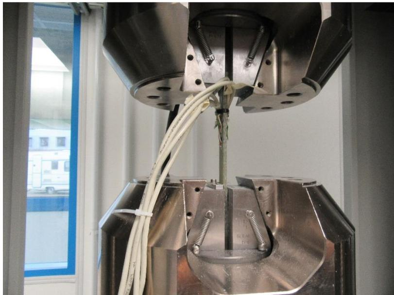
Figure C- 1: Tensile test set-up (1)
