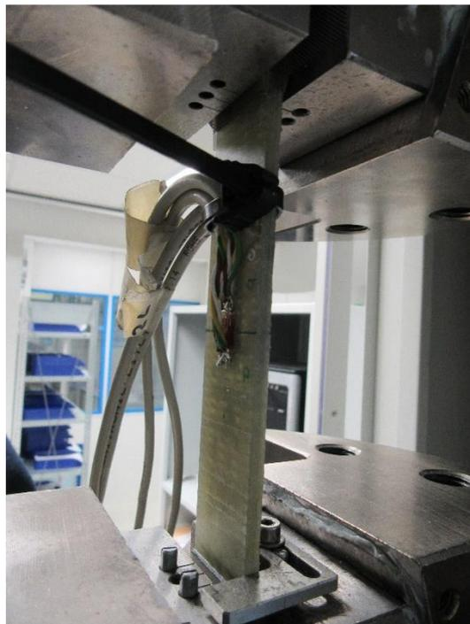
Figure C- 2: Tensile test set-up (2)
