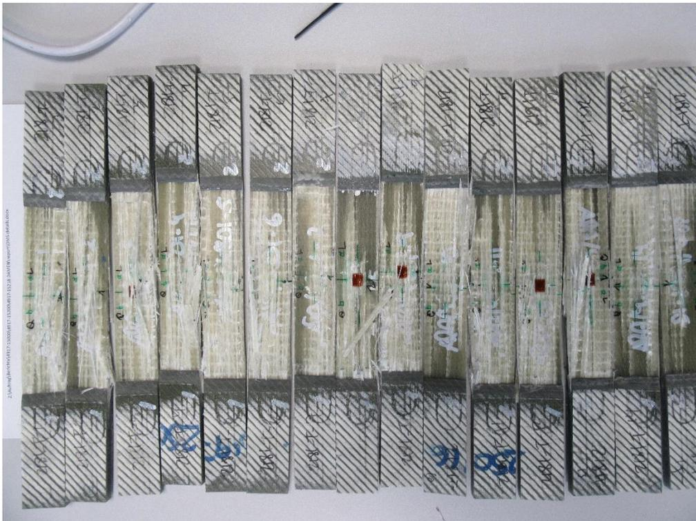
Figure E-1: Broken tensile coupons, fibers at 0°, Top view
