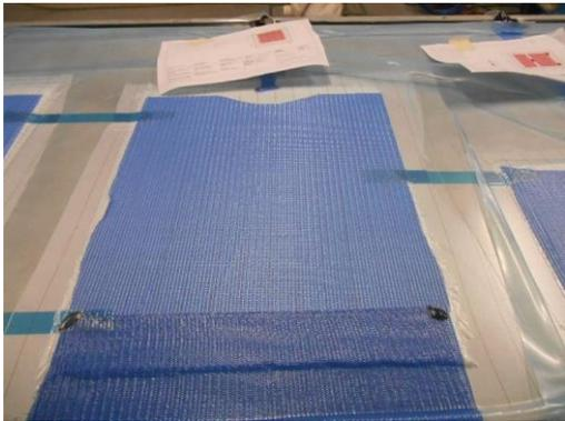
Figure B- 3: Dry fiber mat, fibers at 90°
