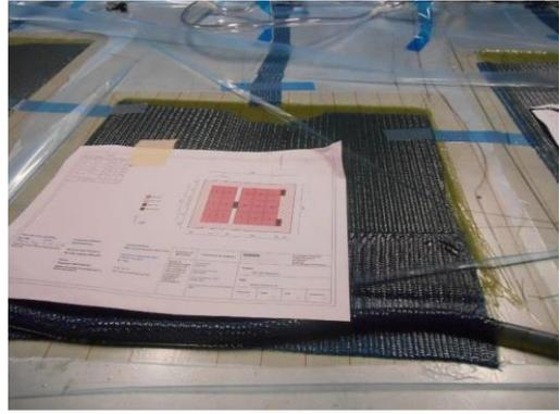
Figure B- 8: Resin transfer finished, Case: Fibers at 0°/90°
