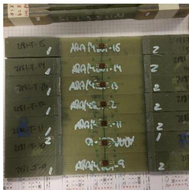
Figure B- 20: Random Tensile Coupons, mounted gauges
