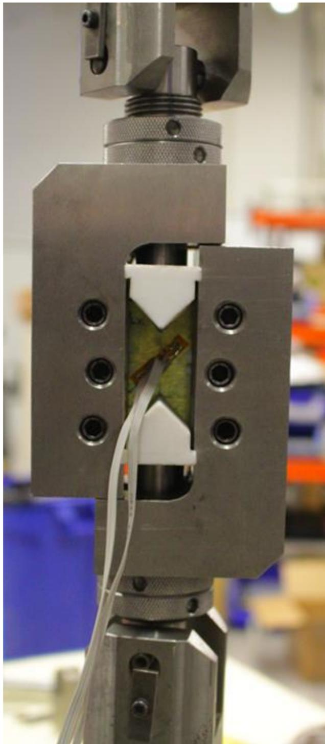
Figure C- 5: Shear tests, set up
