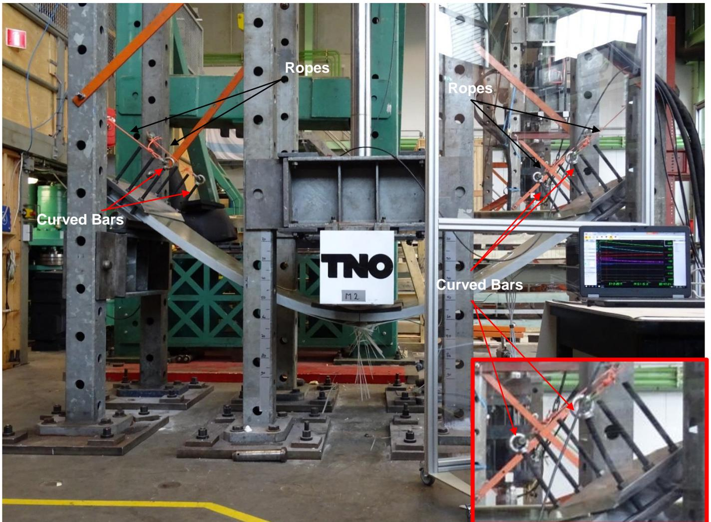
Figure 4-20: Photo of 2<sup>nd</sup> monolithic panel before it was unmounted from the testing frame, obvious introduction of horizontal forces
