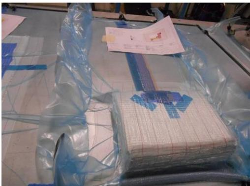
Figure B- 5: Dry fiber mat, thick panel, fibers at 0°
