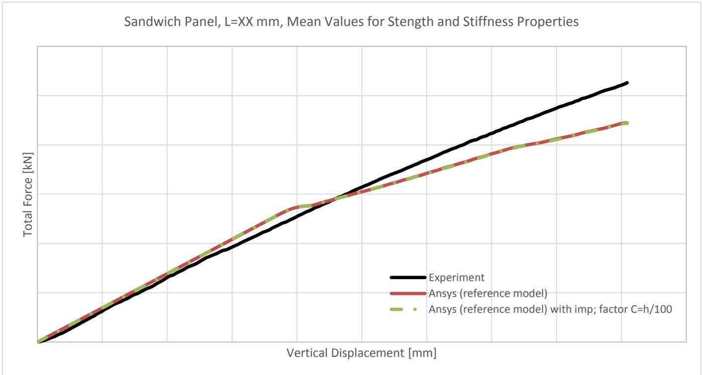
Figure 4-10: Vertical force-displacement curves, 2<sup>nd</sup> sandwich Panel
