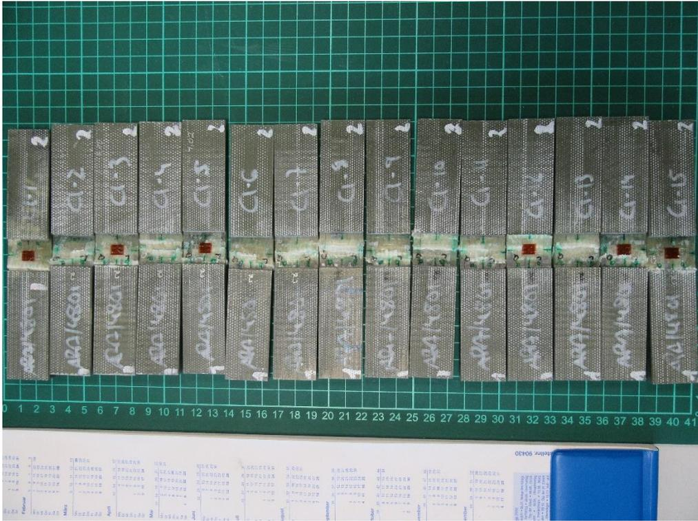
Figure E-5: Broken compressive coupons, fibers at 0°, Top view
