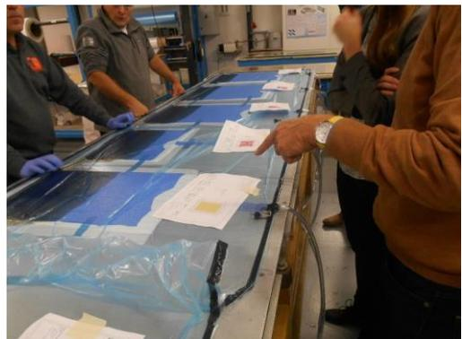
Figure B- 6: Resin transferring, VARTM
