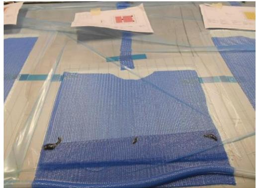
Figure B- 4: Dry fiber mat, fibers at 0°/90°
