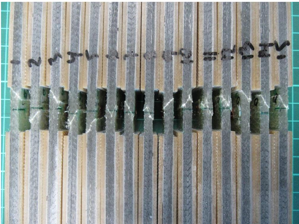
Figure E-8: Broken compressive coupons, fibers at 90°, Top view
