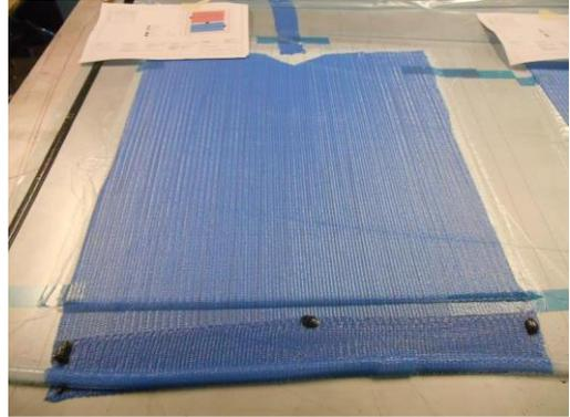
Figure B- 2: Dry fiber mat, fibers at 0°
