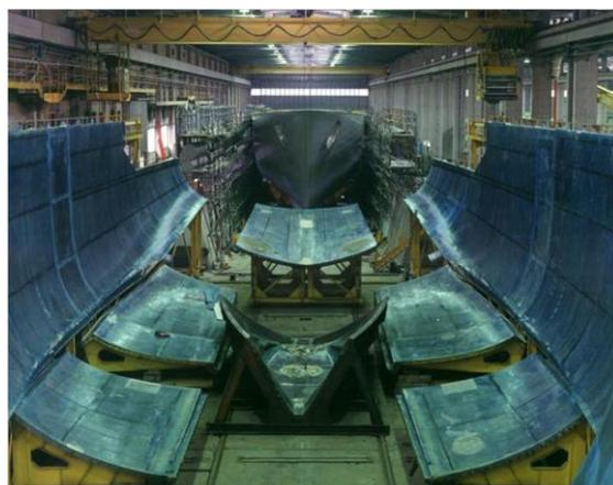
Figure 6-10: Steel hull mould (in segments)
