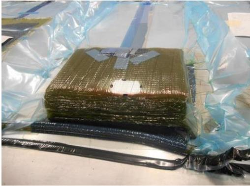
Figure B- 9: Resin transfer finished, Case: thick panel
