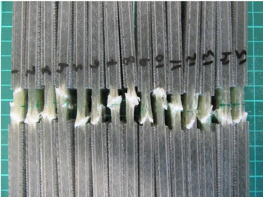
Figure E-6: Broken compressive coupons, fibers at 0°, Side view
