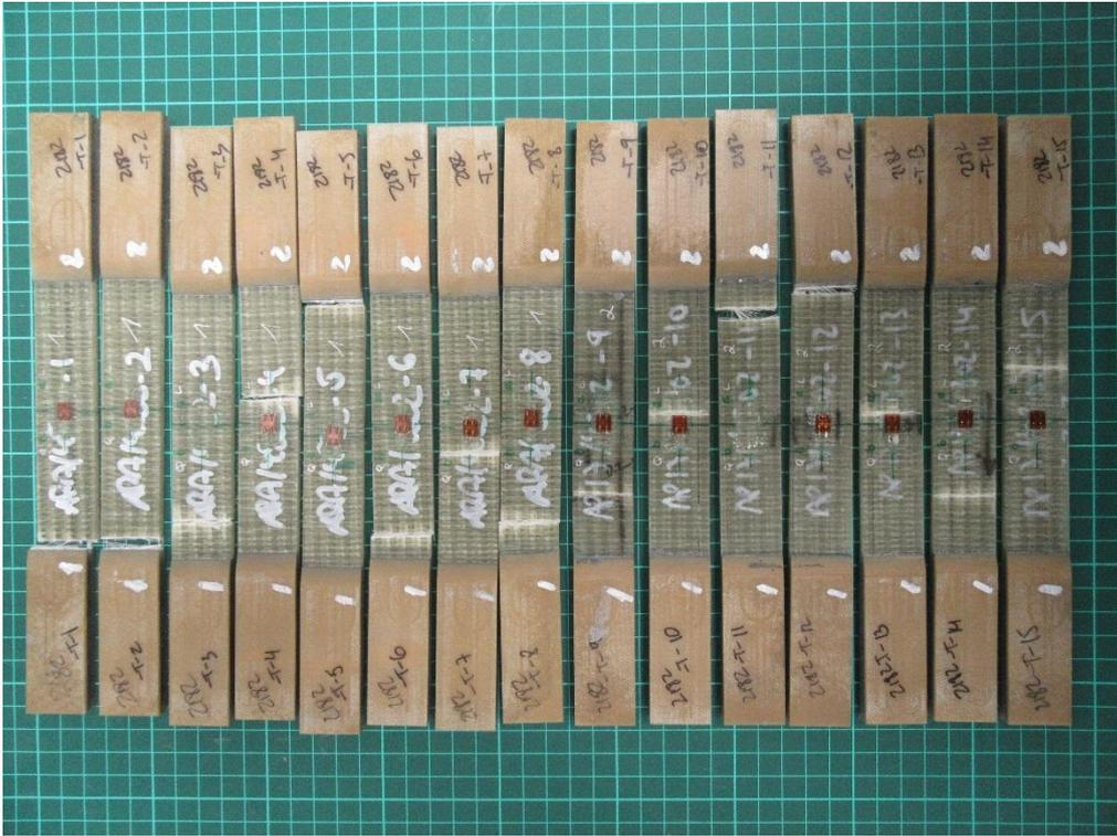
Figure E-3: Broken tensile coupons, fibers at 90°, Top view
