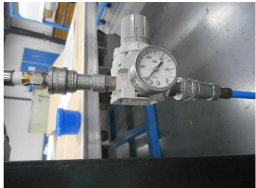
Figure B- 12: Control of underpressure during VARTM
