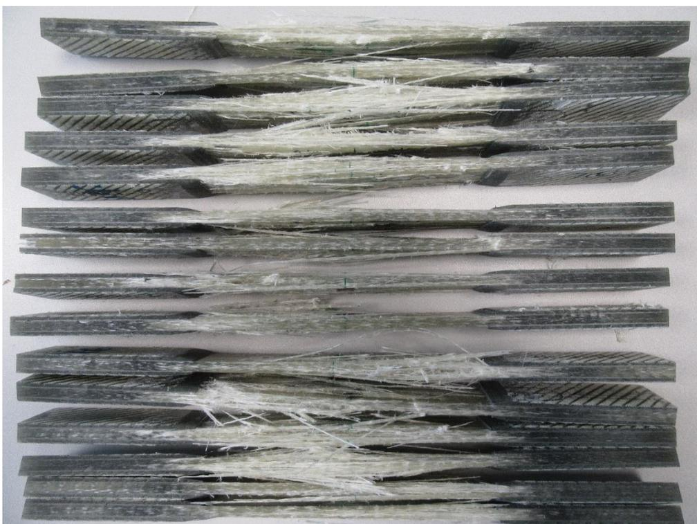
Figure E-2: Broken tensile coupons, fibers at 0°, Side view
