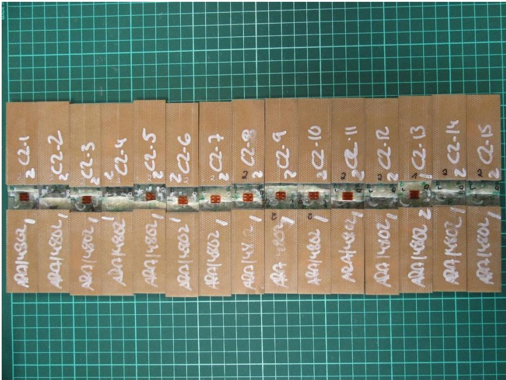
Figure E-7: Broken compressive coupons, fibers at 90°, Top view
