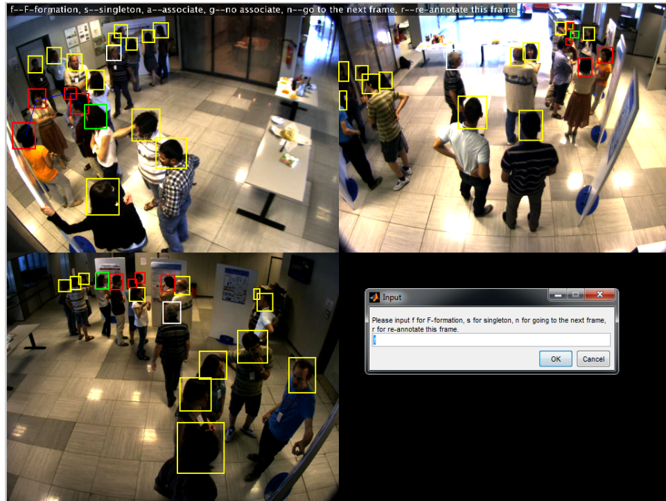
Fig. 4. Example snapshot of the annotation graphical user interface where one F-formation has been annotated for. Labelled F-formation full members, associates, and singletons are indicated by red, green and white boxes respectively. The blue lines (top right frame) between the red boxes indicate which F-formation the full members belong to.
