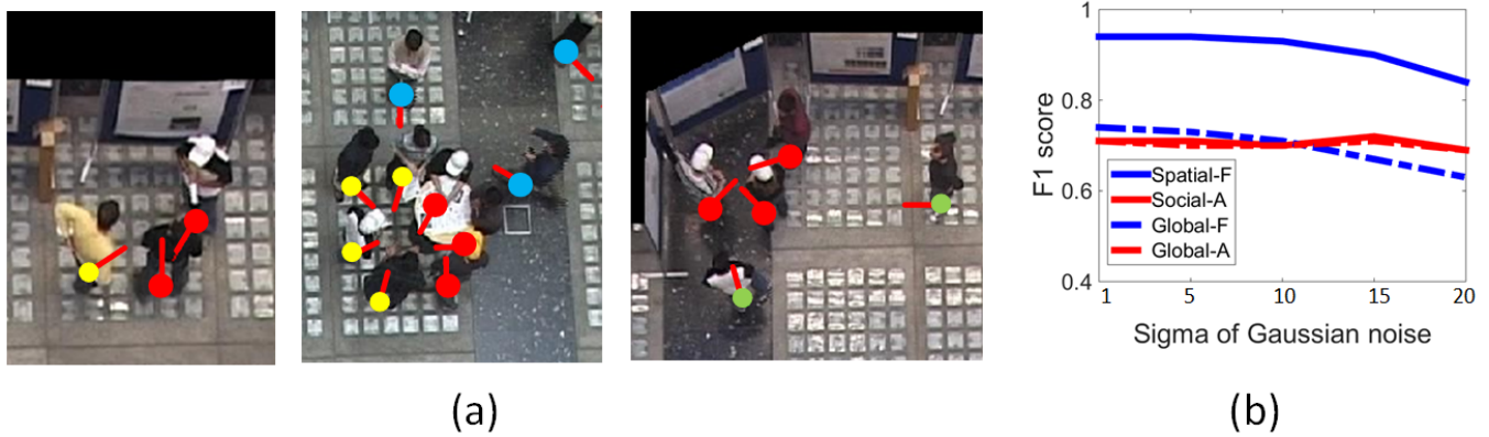
Fig. 8. (a): example associate detection results: Red dots - members of an F-formation; red lines - body orientation; yellow dots - correctly detected associates; blue dots - correctly detected singletons; and green dots - missed associate detections. (b): F1 score of F-formation detectors spatial-F and global-F and associates detectors social-A and global-A with noisy test data.
