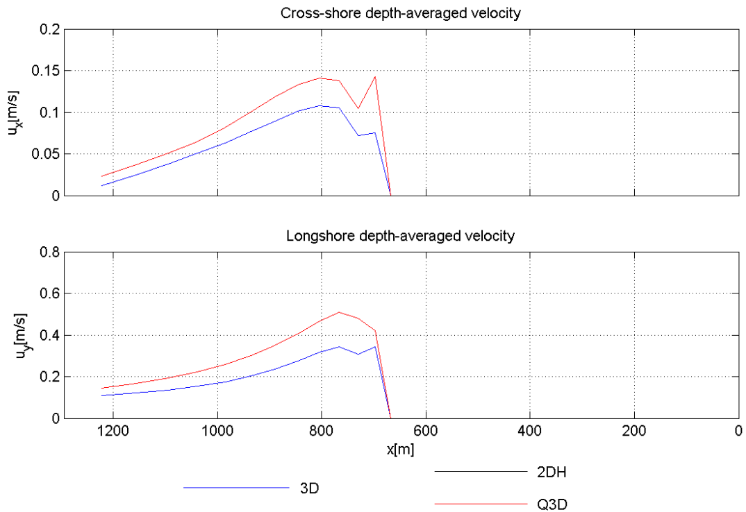
Figure 4.7 Depth-averaged cross-shore and longshore velocities at cross-section BB'
