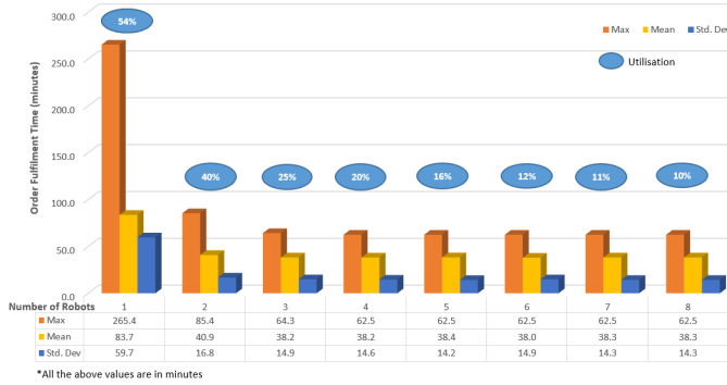
Fig. 8: Order fulfilment time with varying maximum number of robots
