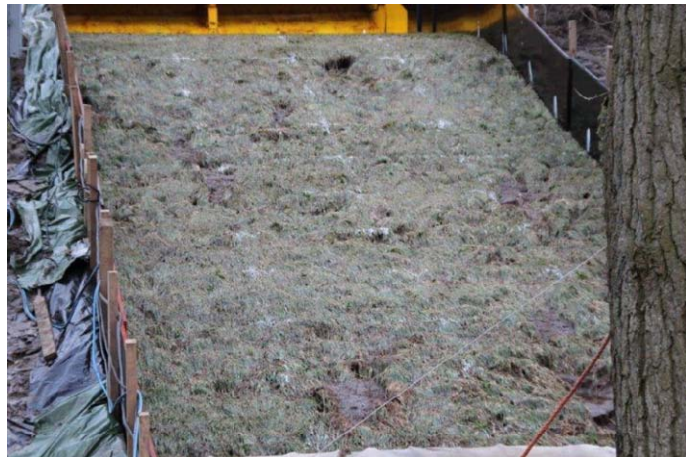
Figure 3.4. Non-failure after testing
