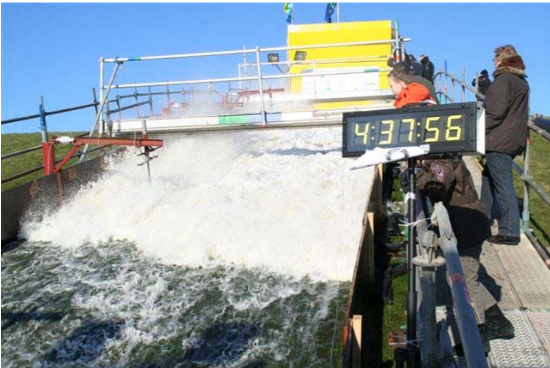
Figure 1.3. Release of a large overtopping wave volume.
