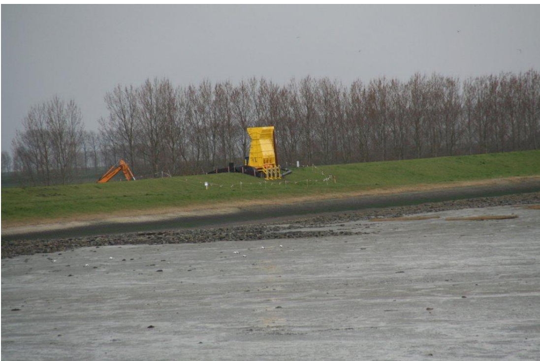
Figure 2.7. Kattendijke - Eastern Scheldt. View on the seaward side, including the Wave Overtopping Simulator which is testing the landward side.
