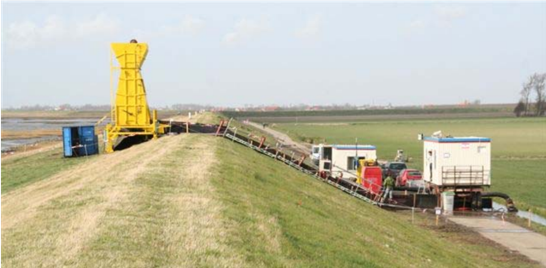
Figure 1.2. Wave Overtopping Simulator on a real dike.
