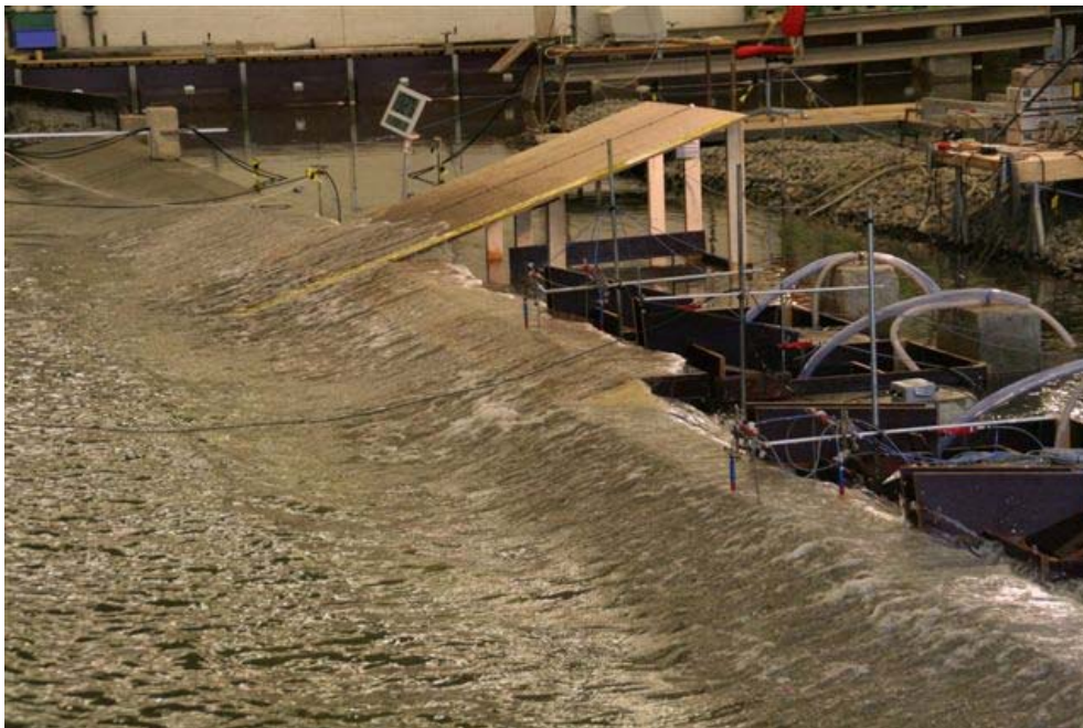
Figure 5.1. Test set-up in Flowdike I on measuring wave run-up and overtopping.
