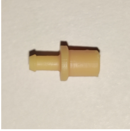
Fig. 7: One of the 12 3D-printed pins that connect the actuation unit with the input air tubes coming from the control unit. A tube fits over one side (left in the Figure) and the other side (right in the Figure) fits in the actuation unit.
