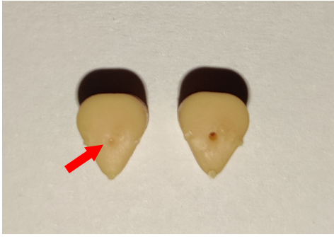
Fig. 14: Two 3D-printed parts. On the left: the part after 3D printing, washing, and curing. The red arrow indicates where the 0.5 mm diameter hole was supposed to be. Due to clogging, only a small part of the hole was successfully printed. On the right: the same part after drilling the hole with a 0.5 mm drill.
