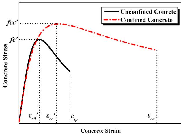
Fig. 9. Stress-strain curves for unconfined and confined concrete.
