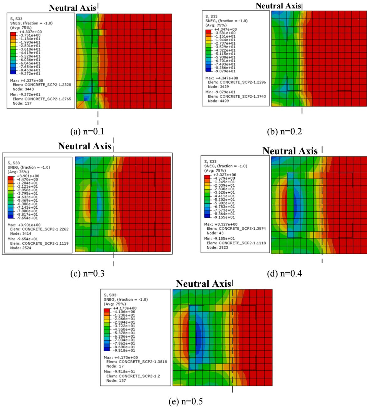
Fig. 23. Normal stress cloud image of cross-section at column bottom with different axial compression ratio.
