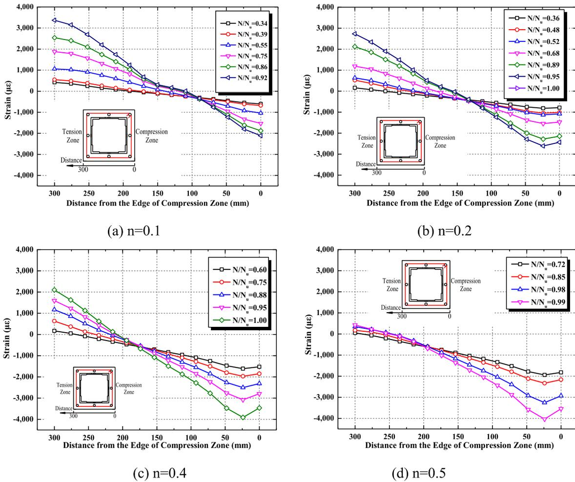
Fig. 25. Concrete strain distribution along cross-section with different axial compression ratio.
