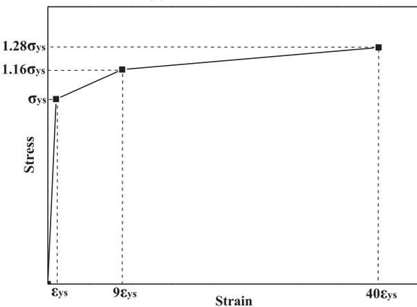
(b) Reinforced steel bar
