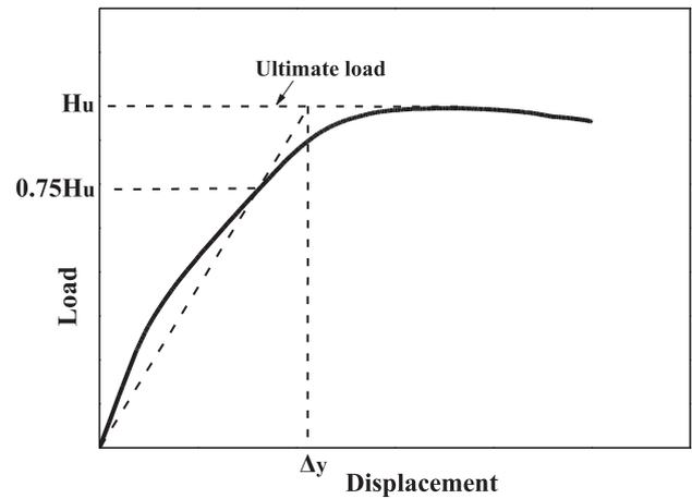
Fig. 14. Definition of displacement ductility ratio.
