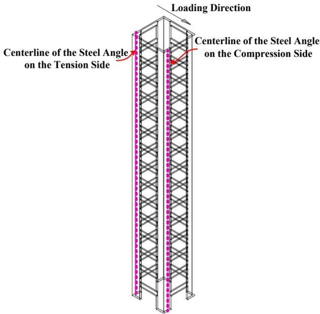
Fig. 29. Stress extraction at centerline of the steel angle on tension and compression sides.
