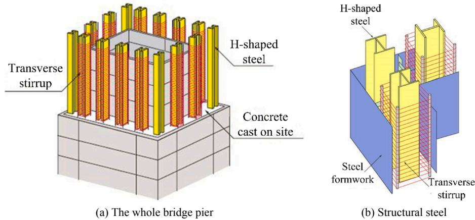
Fig. 1. Hybrid hollow high (3H) pier [1].
