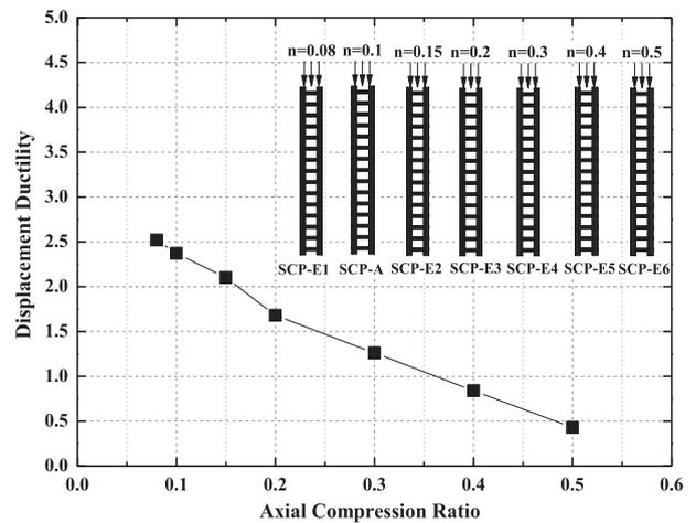
Fig. 21. Displacement ductility of specimens with different axial compression ratio.
