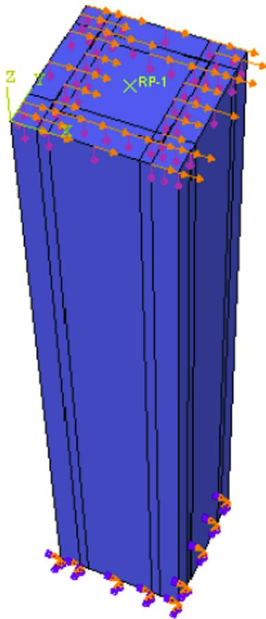
Fig. 12. Boundary condition and load application.
