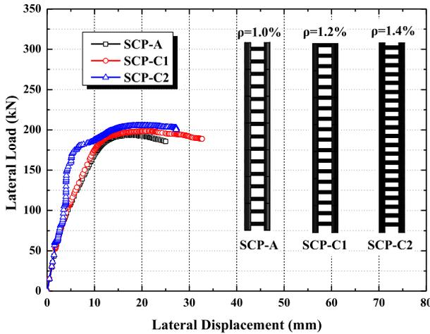
Fig. 16. Lateral load-displacement curves of specimens with different steel-plate hooping ratio.
