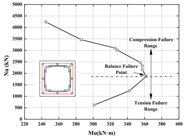
Fig. 22.  $N_u - M_u$  curve of composite columns under different axial compression ratio.
