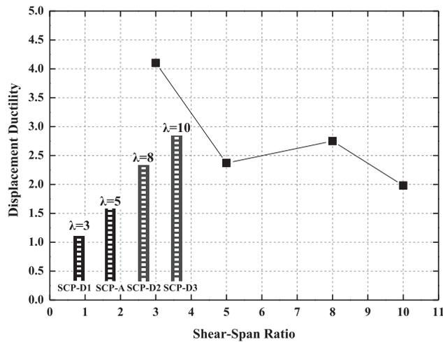
Fig. 19. Displacement ductility for specimens with different shear-span ratio.
