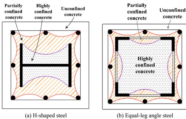
Fig. 6. Confinement zones in concrete encased steel composite columns.
