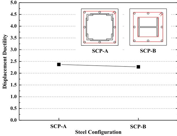
Fig. 15. Displacement ductility of specimen SCP-A and SCP-B.
