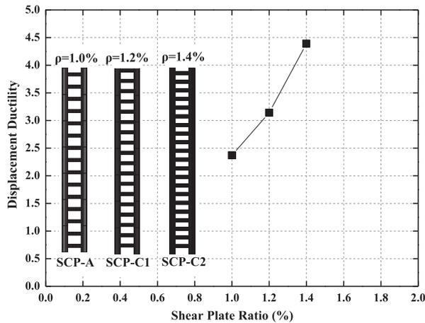
Fig. 17. Displacement ductility for specimens with different steel-plate hooping ratio.
