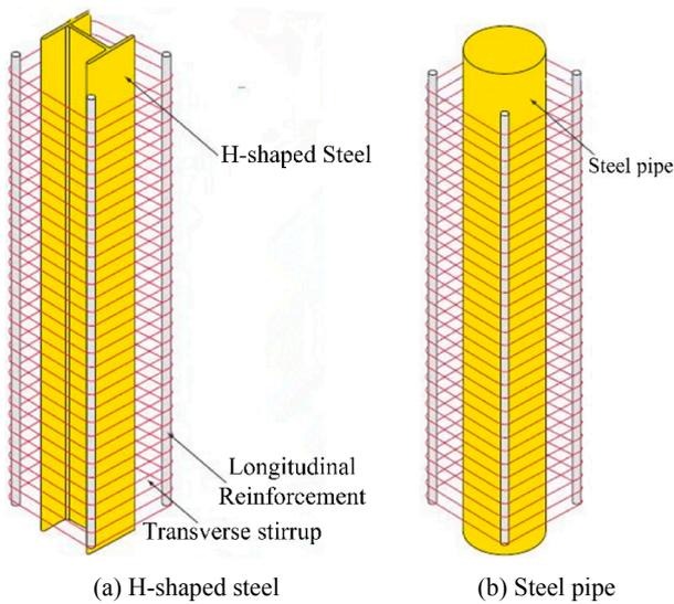
Fig. 2. Steel types in hybrid hollow high (3H) pier.
