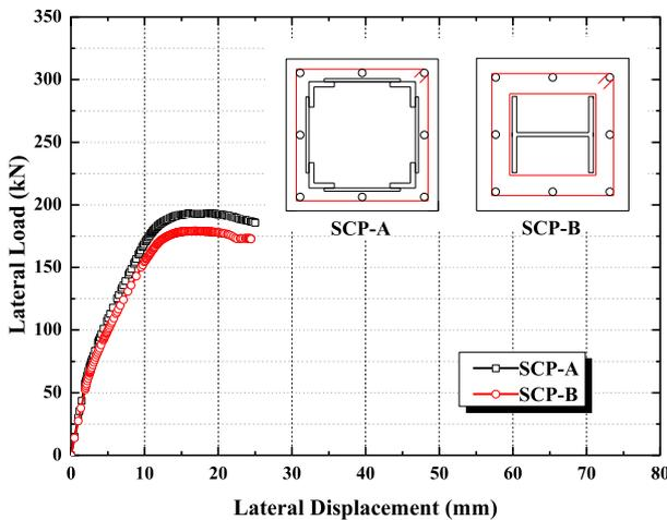
Fig. 13. Lateral load-displacement curves of specimen SCP-A and SCP-B.
