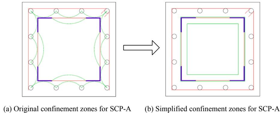
Fig. 8. Confinement zones for SCP-A.
