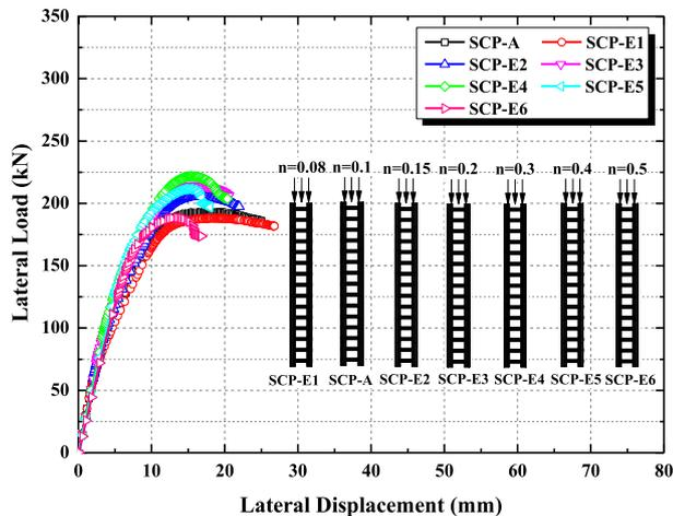
Fig. 20. Lateral load-displacement curves of specimens with different axial compression ratio.
