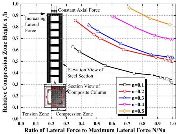
Fig. 24. Relative compression zone height of section at column bottom.
