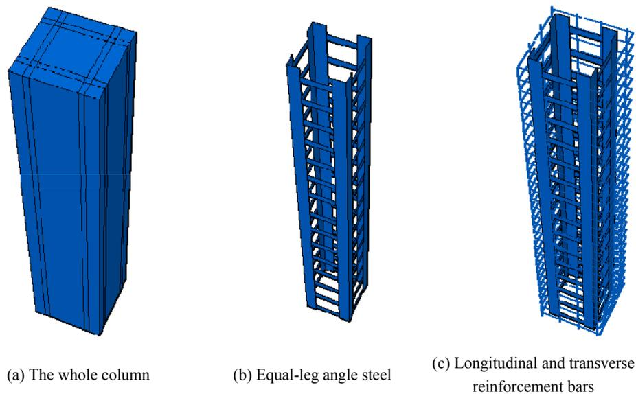
Fig. 5. Finite element modelling for the concrete encased equal-leg angle steel composite column.
