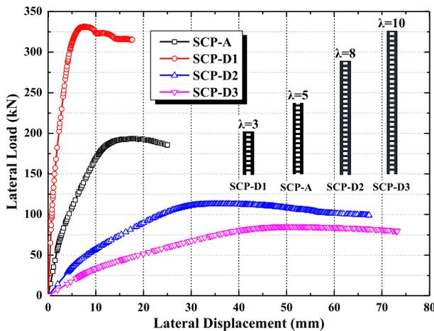
Fig. 18. Lateral load-displacement curves of specimen with different shear-span ratio.
