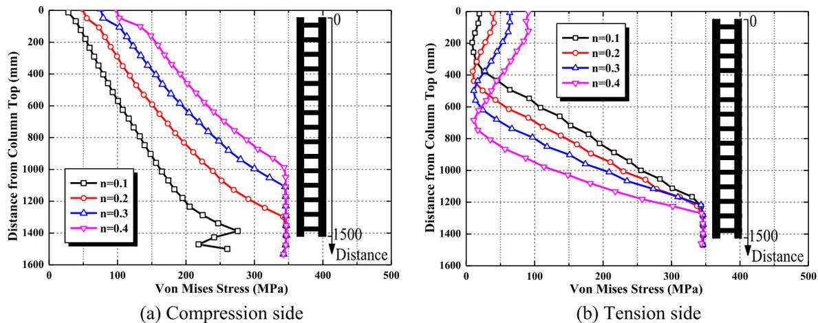
Fig. 32. Von Mises stress of SCP-G3 under different axial compression ratio.
