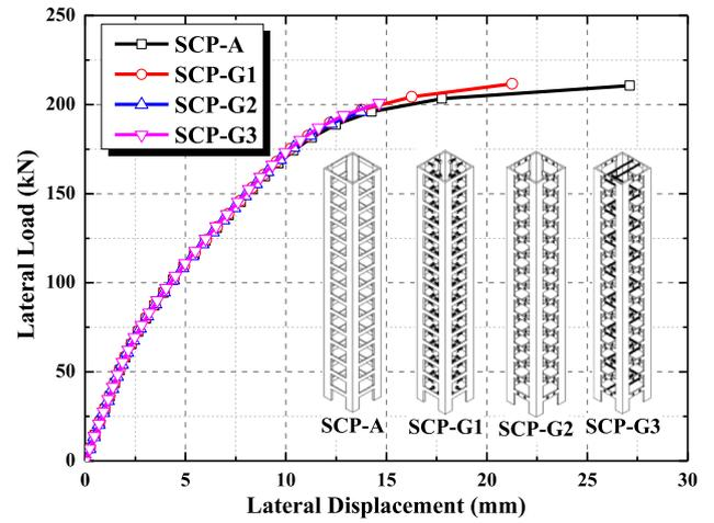
Fig. 28. Lateral load-displacement curves of SCP-A and SCP-G1 ~ G3.
