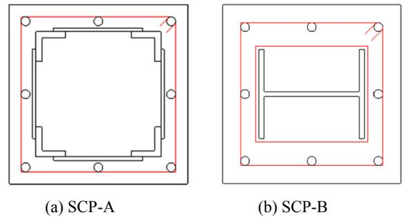
Fig. 4. Cross section of specimens SCP-A and SCP-B.
