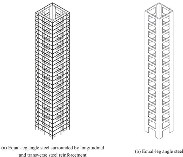
Fig. 3. Equal-leg angle steel and reinforcing bars.
