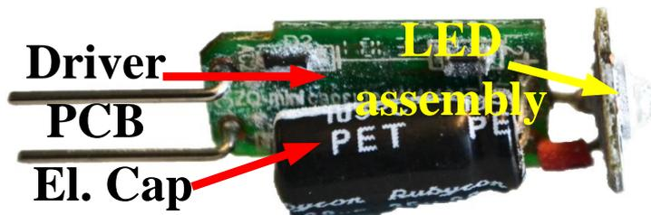
**Figure 3.8:** Philips G4 capsule PCB layout.
