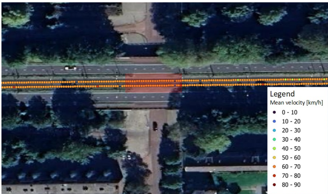
Figure 4.38: Mean velocity tramway transition zone Brug 717 in 2022. The bridge has been shaded with red.
