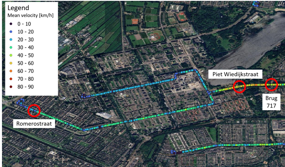
Figure 4.7: Overview of the three proposed locations with the mean velocities of the trams in 2021.
