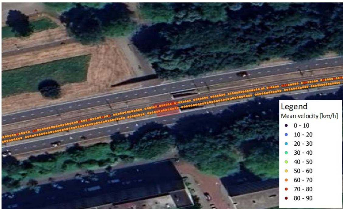
Figure 4.36: Mean velocity tramway transition zone Piet Wiedijkstraat in 2022. The bridge has been shaded with red.
