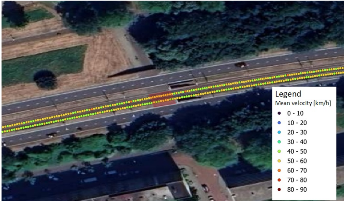
Figure 4.35: Mean velocity tramway transition zone Piet Wiedijkstraat in 2021. The bridge has been shaded in red.
