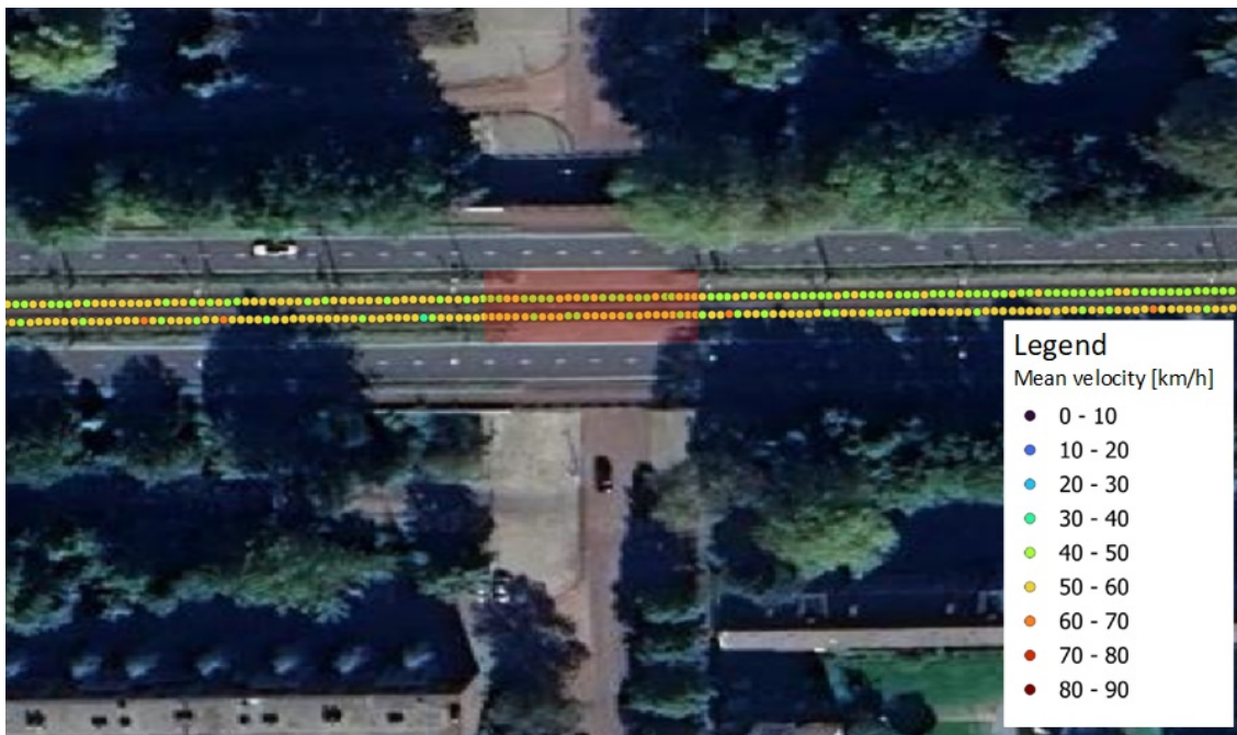
Figure 4.37: Mean velocity tramway transition zone Brug 717 in 2021. The bridge has been shaded with red.
