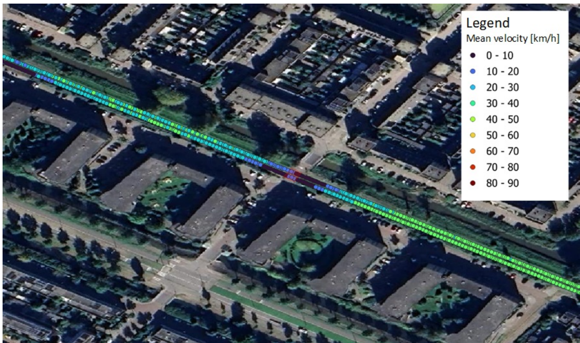
Figure 4.40: Mean velocity tramway transition zone Romerostraat in 2022. The bridge has been shaded in red.
