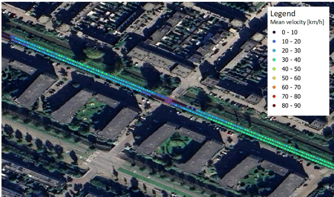
Figure 4.39: Mean velocity tramway transition zone Romerostraat in 2021. The bridge has been shaded in red.
