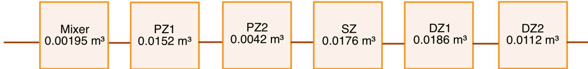
Figure 3.1: Schematic of the individual volumes used by Telidevara [8].
