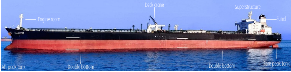
Figure 2.2: Tanker with labeled hull points (adapted from Source: [31])
