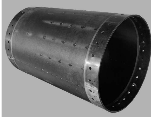
Figure 8.4: Cylinder layout before application of the speckle pattern
