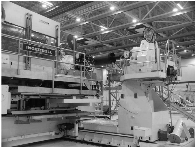
Figure 2.1: General view of an Ingersoll AFP machine (photo: Boeing)
