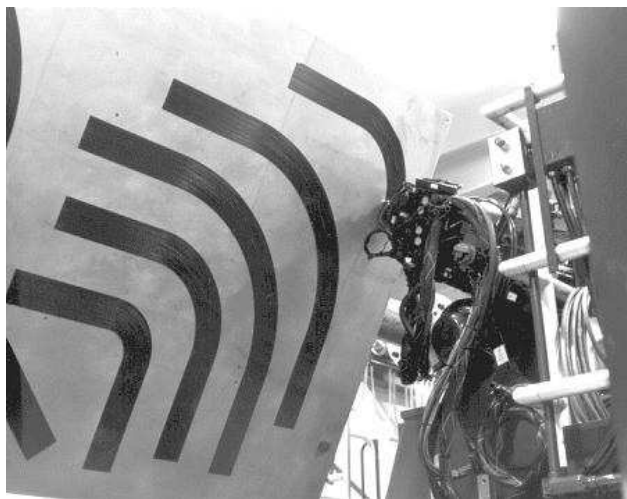
Figure 1.5: Steered fibers laid down by an advanced fiber placement machine (photo: IMT)
