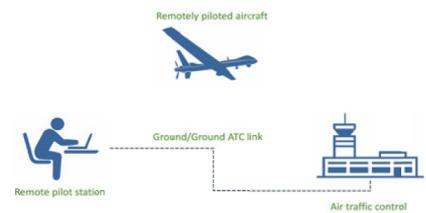
Figure 4.23: Ground via communications service provider [4]
